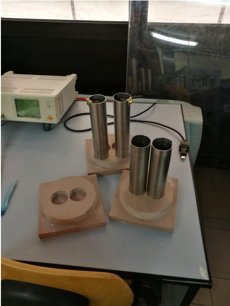
Figure 3.12: Real prototype with electrodes of 200 mm and distance  $d = 2$  mm
