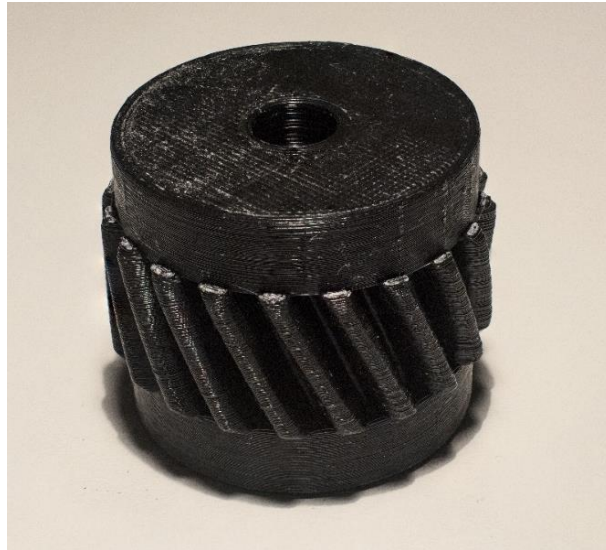
Figure 32 Gear wheel produced without grooves and internal supports
