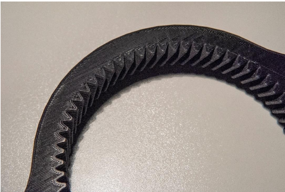
Figure 54 Detail of the teeth profile obtained with the first attempt
