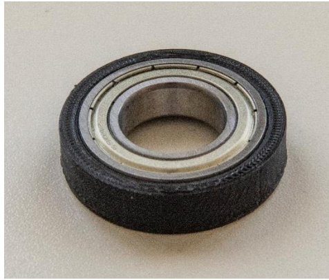
Figure 49 Coupling of a bearing with the PLA outer ring
