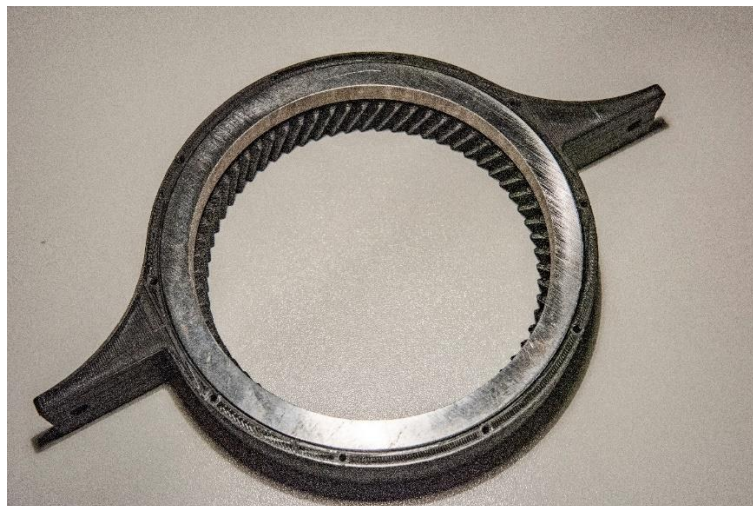
Figure 56 Final structure of the side crown, coupled with the steel ring
