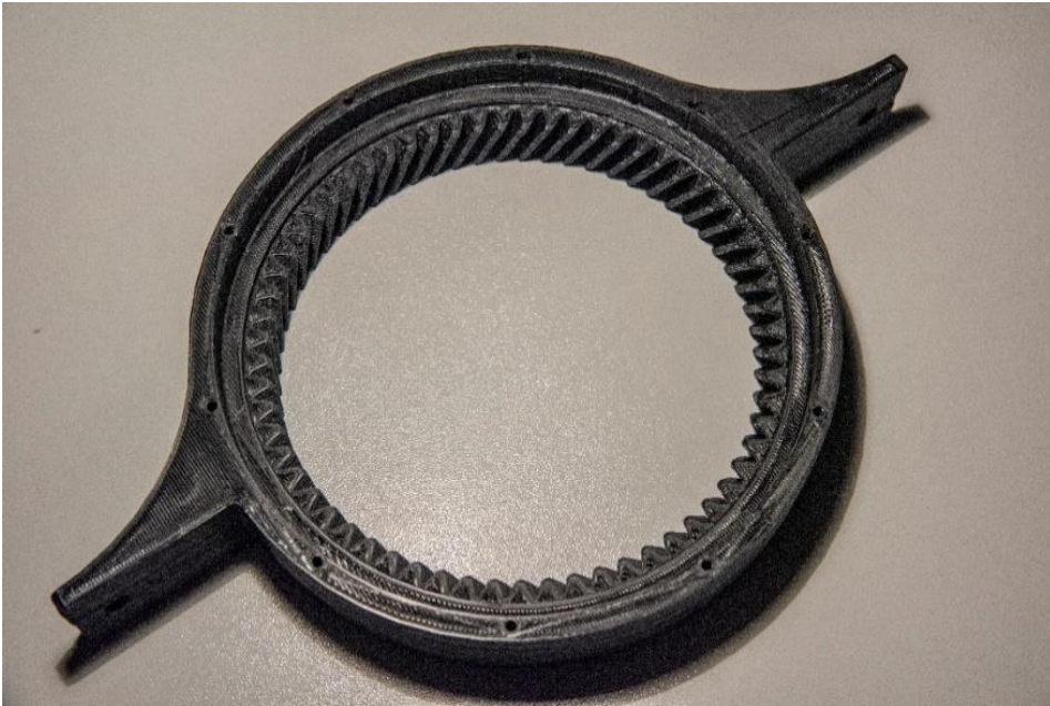
Figure 53 First printing result of the lateral internal gear
