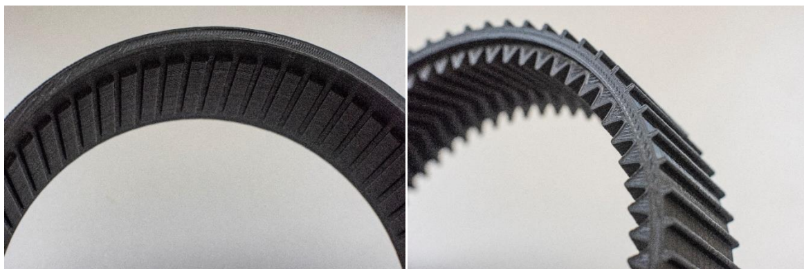
Figure 60 Detail of the coupling between the outer part and the inner part with the double-helical toothing
