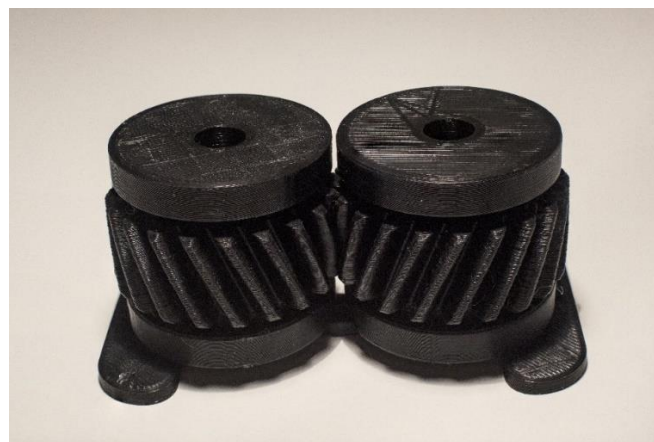
Figure 38 Final result of the meshing test, with contact of the adjacent flanges
