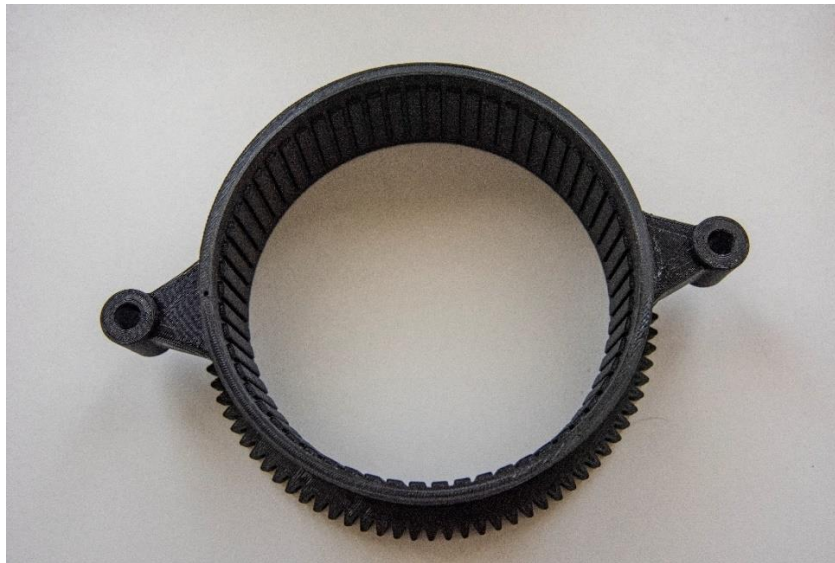
Figure 59 Final result of the coupling between the outer component and the side elements
