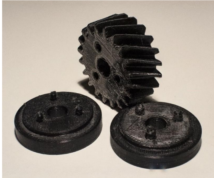
Figure 33 Structure of the gear wheel divided into three components
