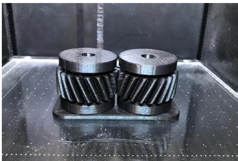
Figure 37 Second meshing test, to have contact between adjacent flanges
