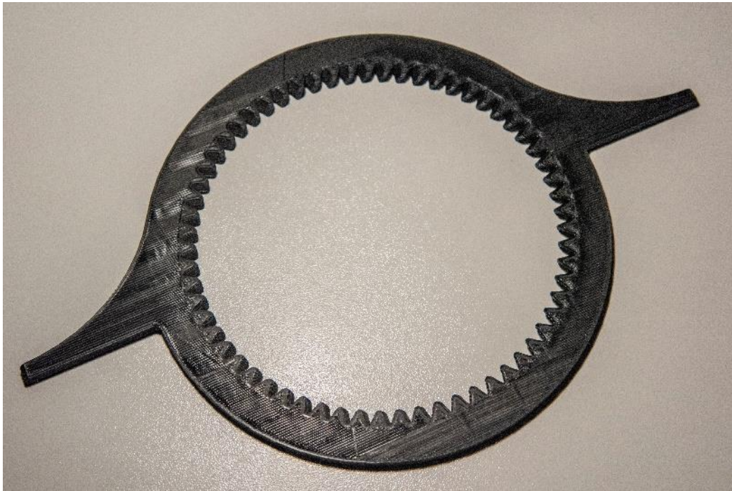
Figure 46 Test tothing that reproduces the internal gear
