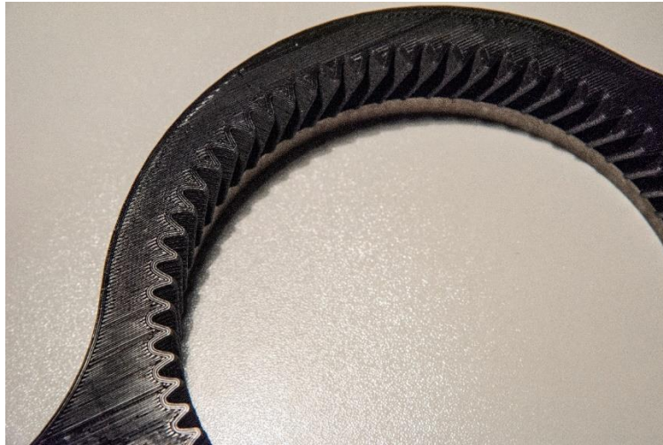
Figure 55 Profile of the teeth obtained in the second attempt, following the narrowing of the profile
