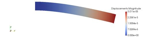
Figure 6.4: Displacements of the eight-layer beam
