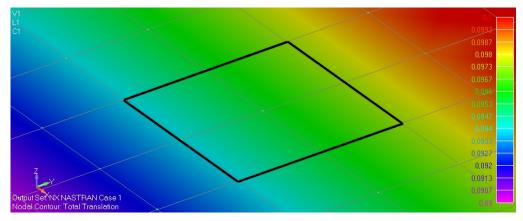
(a) Displacements on the mid span local zone obtained by Nastran
