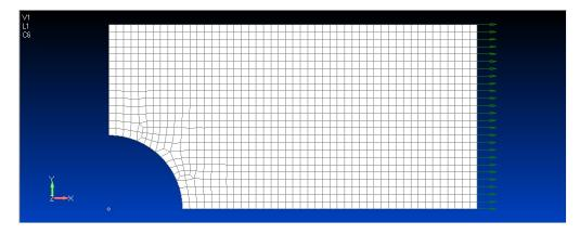
Figure 7.7: Plate hole mesh structure
