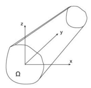
Figure 1.1: Beam reference system
