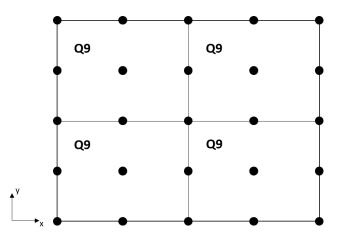
Figure 3.9: Structural mesh - 4Q9
