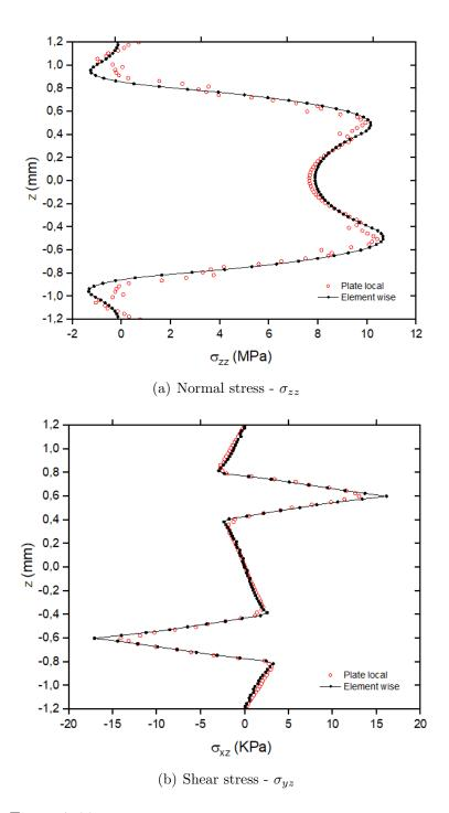
Figure 7.22: Normal and shear stresses out plane in the free-edge
