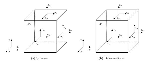
Figure 1.3: Stress and Deformation components
