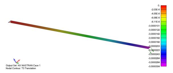
Figure 6.6: 2D eigth layer beam z displacements.
