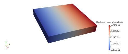
(b) Displacements on the mid span local zone obtained by CUF (Mul2 code)
