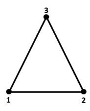
Figure 2.4: Three-node linear L3 element
