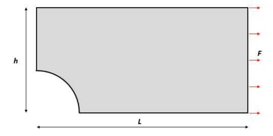
Figure 7.6: Plate hole reduced model
