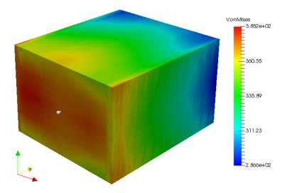
Figure 7.12: Plate hole Von Misses stresses in the most critical element
