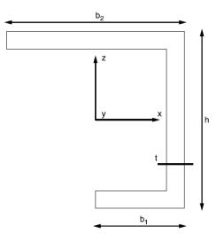
Figure 6.1: C section geometry.
