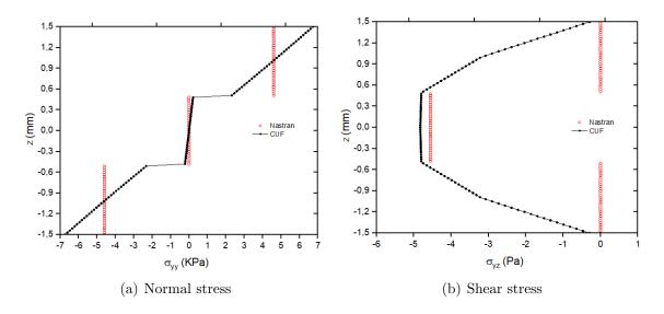
Figure 7.4: Normal and shear stress distribution along the z-axis at mid span
