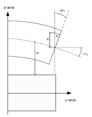
Figure 1.4: EBBT model of deformations
