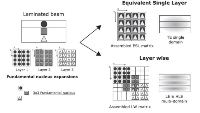
Figure 3.7: Assembly procedure of the stiffness matrix through ESL and LW approaches, *Source*: [6]
