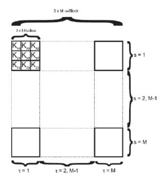
Figure 2.7: Assembly of the  $\tau - s$  sub-matrix
