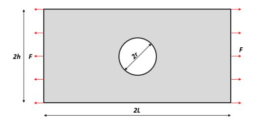
Figure 7.5: Plate hole model and geometrical features
