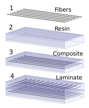
Figure 3.3: Example of a composite laminate
