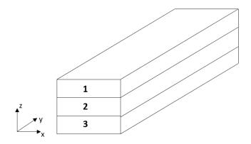
Figure 3.4: Generic composite laminate beam
