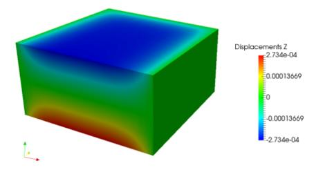
Figure 7.11: Plate hole displacements in z direction of the most critical element
