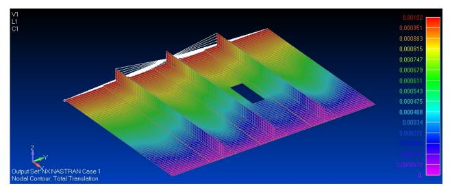
Figure 7.14: Wing structure displacements
