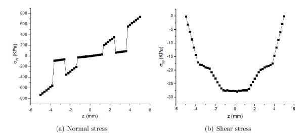
Figure 6.5: Normal and shear stress distribution along the z-axis at mid-span for the eight-layer beam.
