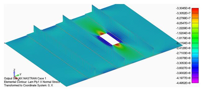
Figure 7.15: Wing structure  $\sigma xx$  stresses at the first layer
