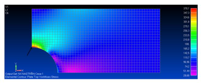
Figure 7.9: Plate hole Von Misses stresses
