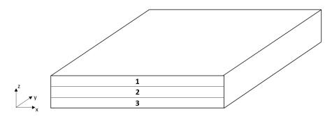
Figure 3.8: Generic composite laminate plate
