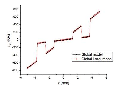
Figure 6.7: Normal stress distribution along the z-axis at mid span
