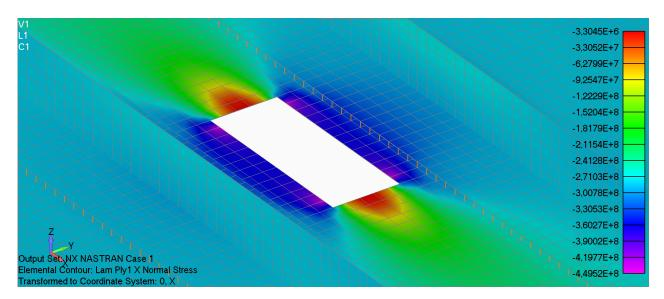
Figure 7.16: Wing structure  $\sigma xx$  stresses around the hole
