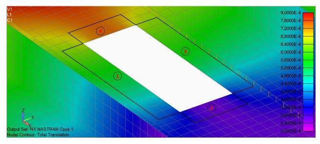
Figure 7.18: Total displacements around the hole
