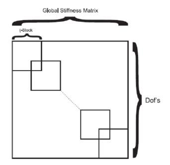
Figure 2.9: Assembly of the global stiffness matrix
