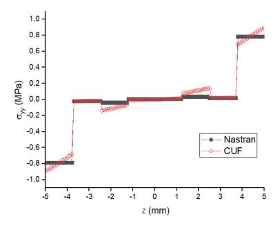
Figure 6.8: Normal stress distribution along the z-axis at mid span
