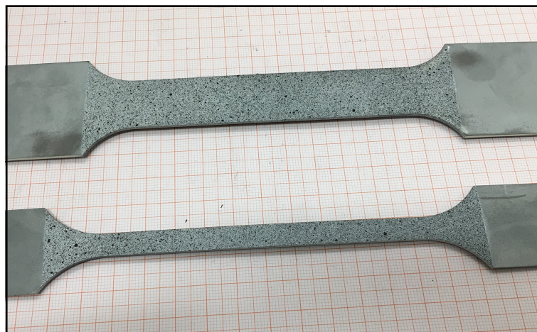
Figure 3.9: Sprayed test specimens
