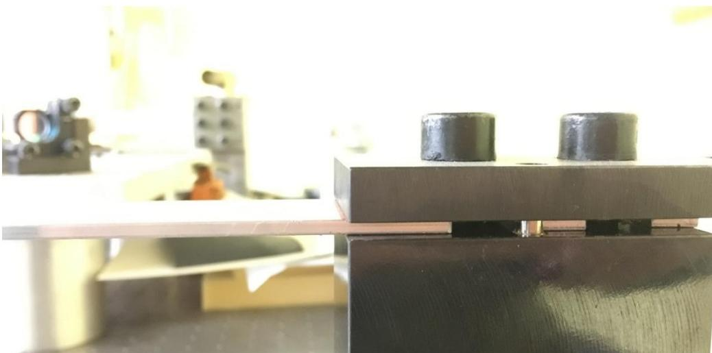
**Figure 30.** Photo of the constraint end of the beam 2 in the rig
