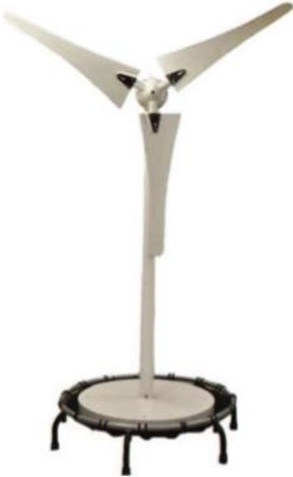
**Figure 12.** The Ampair 600 Wind Turbine test bed
