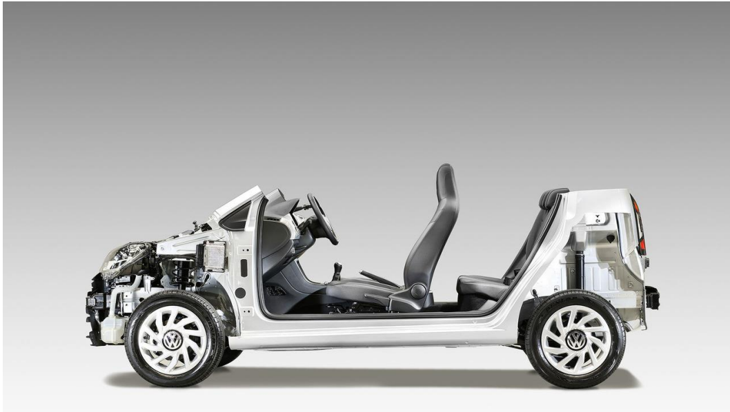
Figure 86: New Small Family (NSF) PQ12 platform (Credit Volkswagen)
