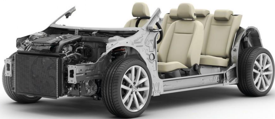
Figure 85: MQB platform for transverse engine vehicle (Credit Volkswagen)
