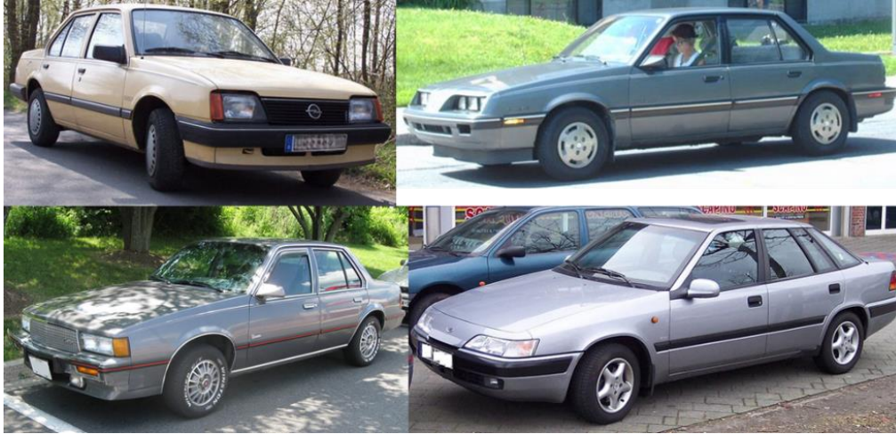
Figure 35: examples of vehicle based on the GM J-platform. On top from left to right: Opel Ascona C 5 , Pontiac Sunbird. On bottom from left to right: Cadillac Cimarron, Daewoo Espero 6 .
