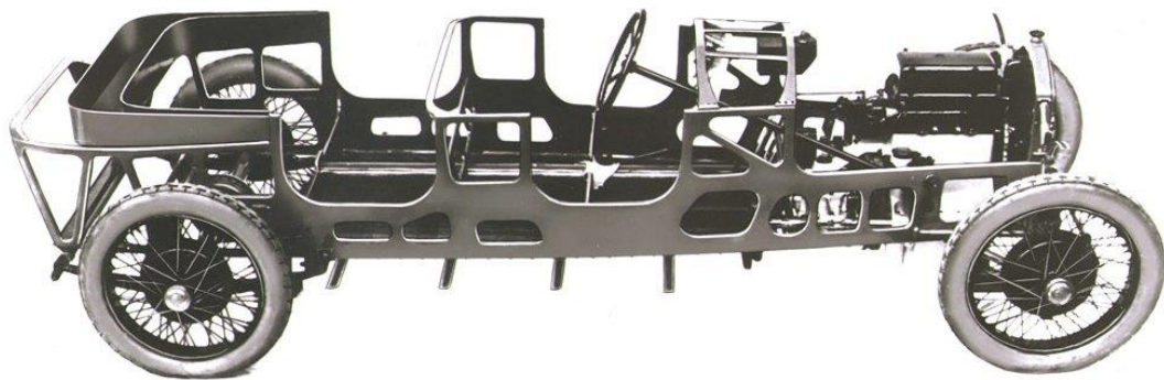
Figure 31: Lancia Lambda, first endeavor of unibody chassis
