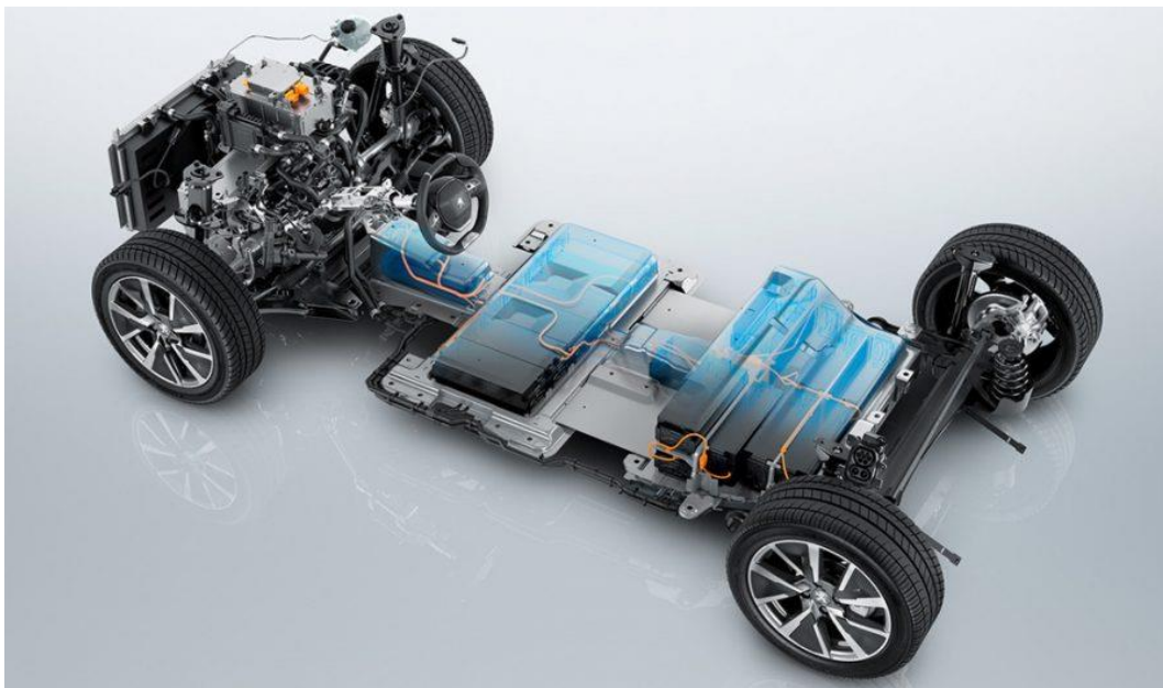
Figure 51: PSA CMP platform for the BEV Peugeot e208 (Credit PSA Groupe)
