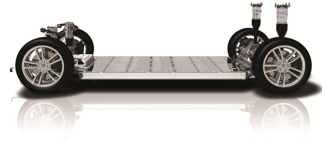
Figure 38: Tesla dedicated BEV platform (Credit Tesla)
