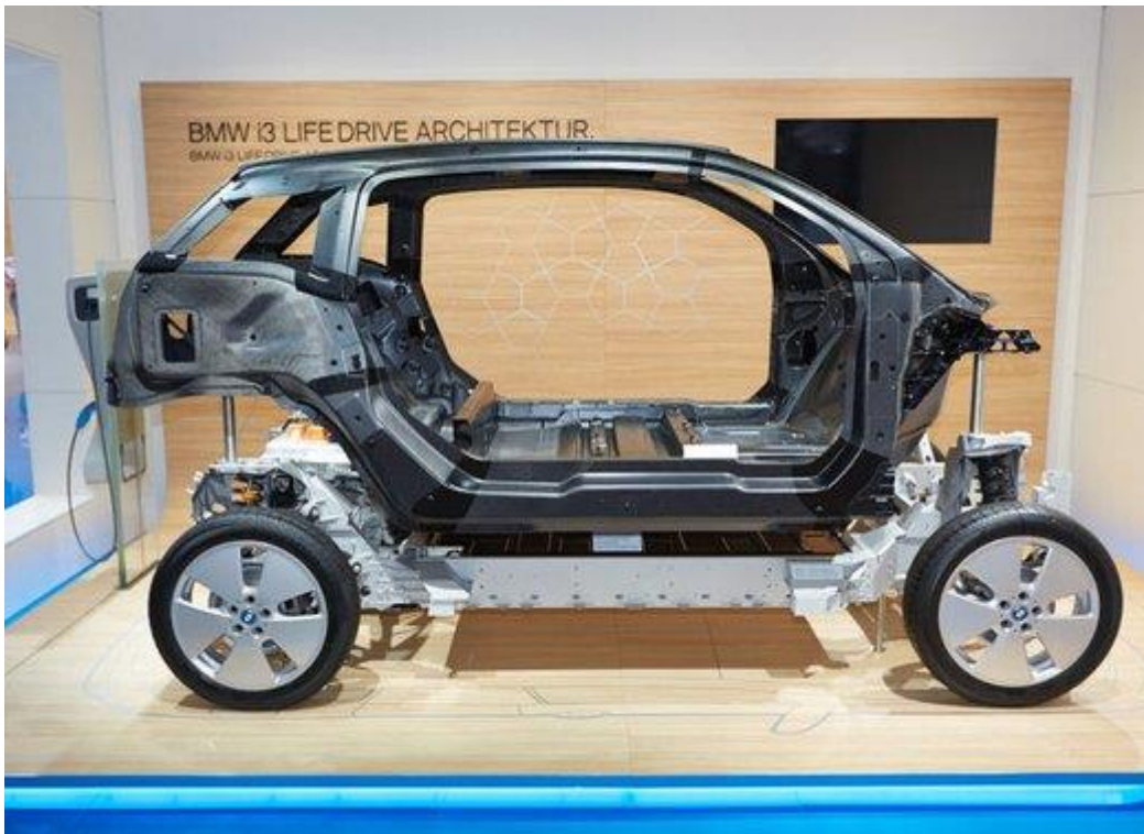
Figure 32: BMW i3 LifeDrive architecture, a modern body on frame design
