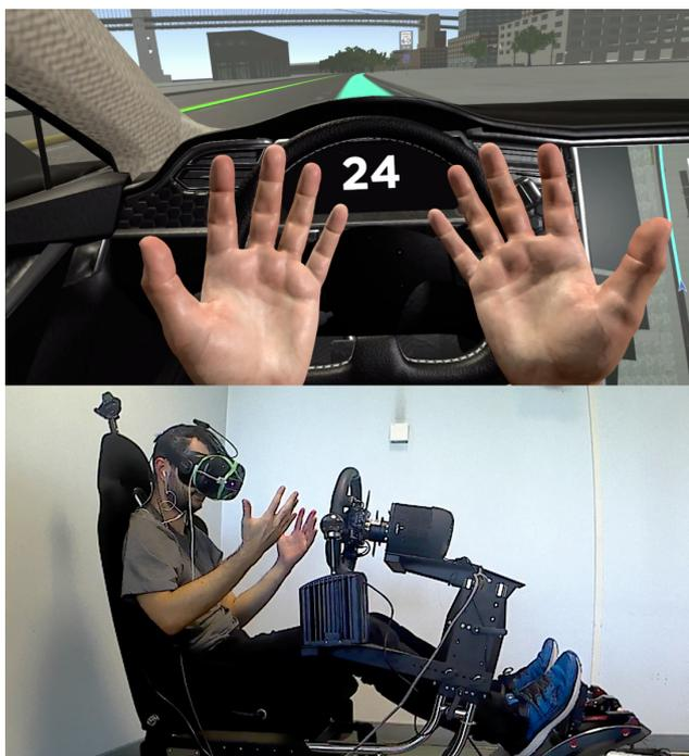
**Figure 4.6:** Leap motion system. At the top the view in VR, at the bottom the outside view [91].
