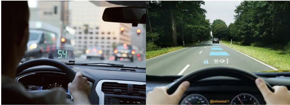
**Figure 2.6:** On the left non contact-analog mode, on the right contact-analog mode[25].
