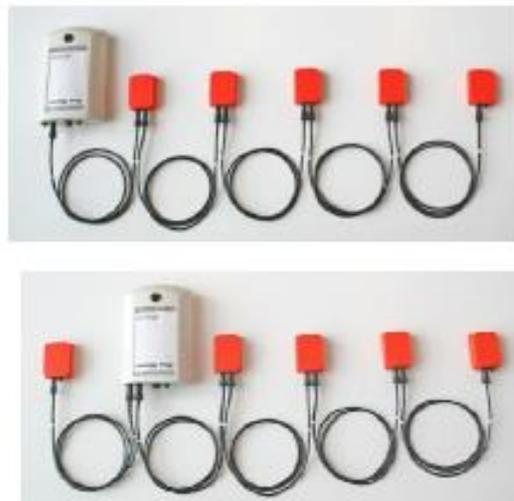
Fig. 2.2.3-2 Motion Trackers connected to Xbus Master (Xsens).
