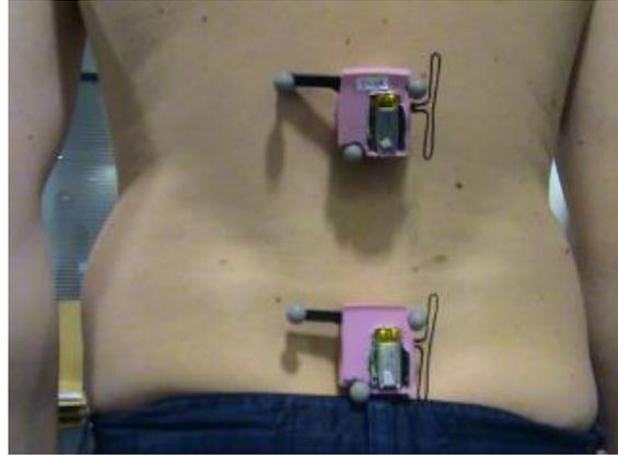
Fig. 1.2.1-6 Sensors placement on lumbar spine (Quantitative assessment of the motion of the lumbar spine and pelvis with wearable inertial sensors, 2010).
