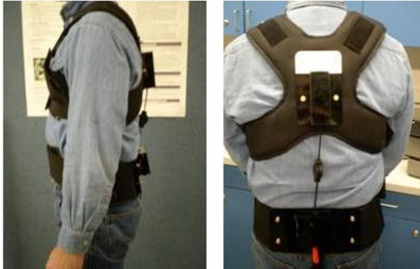
Fig. 1.2.1-11 Industrial Lumbar Motion Monitor (Schall, et al., 2015).
