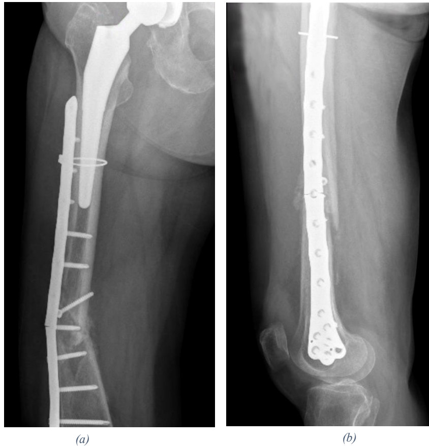
Figure 3.6: Anteroposterior (a) and right-left (b) X-ray views of the plate break
