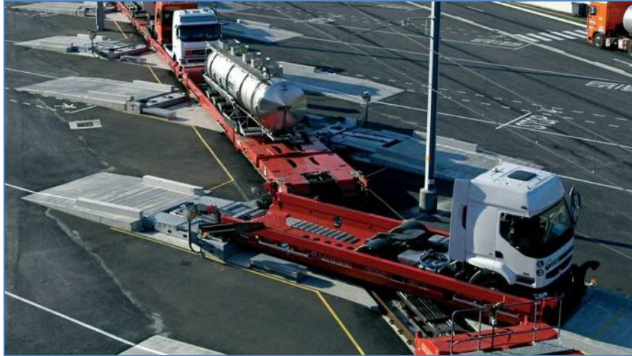
Figure 2-16 Lohr, horizontal loading/unloading technology [19]
