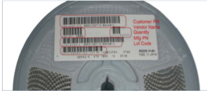
Figure 22. The key to materials management is automating the fool-proof capture of vendor data from the bar codes on the reel and posting this information into the material database.
