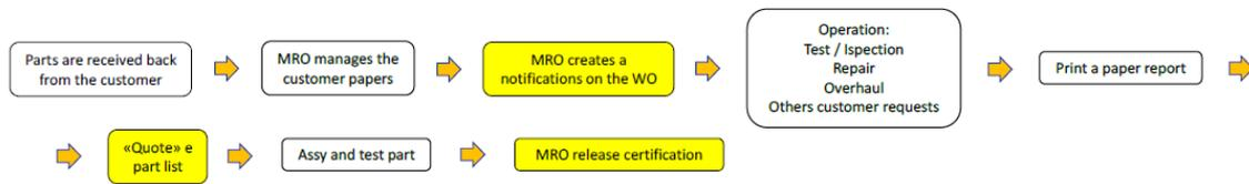
Figura 5.11: *Repair and overhaul process - current state*
