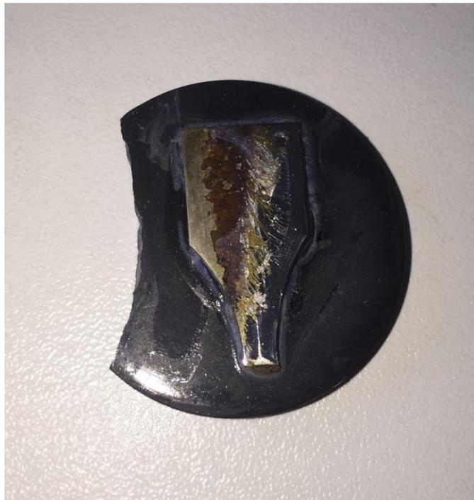
FIGURE 23: EXAMPLE OF FAILED POLISHING IN A TWIP STEEL, DUE TO AN OXIDATION OF THE SURFACE DURING THE VIBRATIONAL POLISHING IN AN OPS COLLOIDAL SOLUTION.
