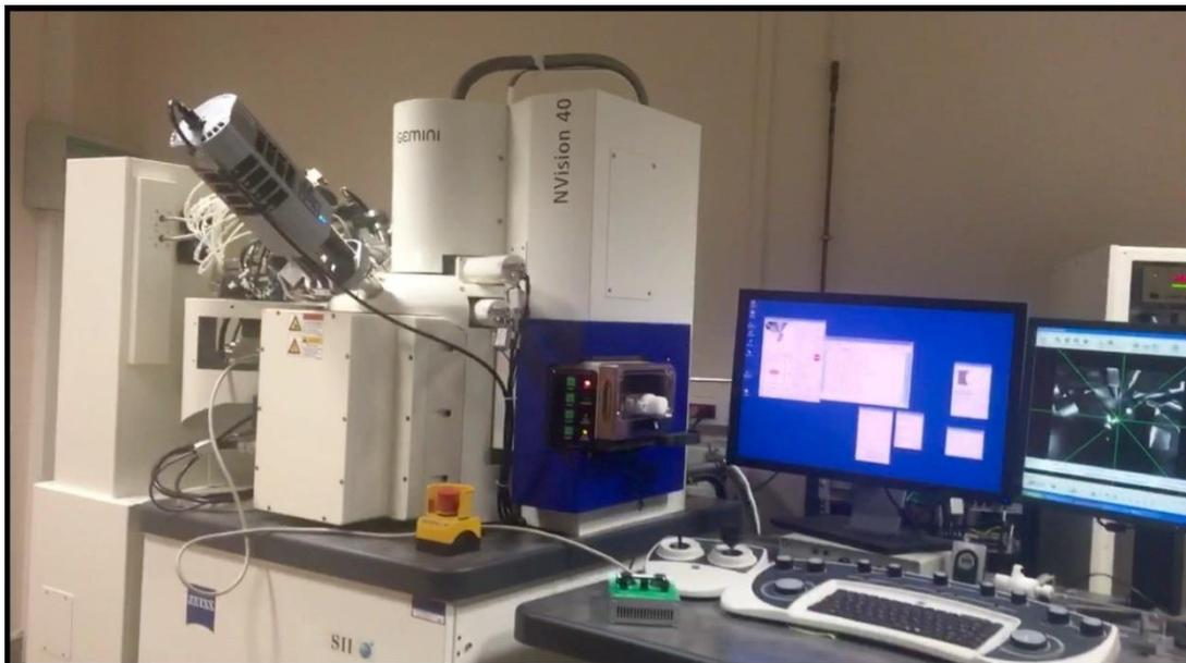
FIGURE 22: IMAGE OF THE FIB SCANNING ELECTRON MICROSCOPE USED IN THIS MASTER'S THESIS.
