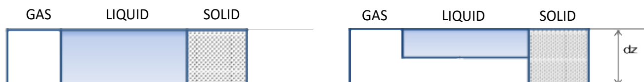
Figure 11: Scheme of complete wetting(left) and partial wetting(right) for the interfaces in a three-phase system
