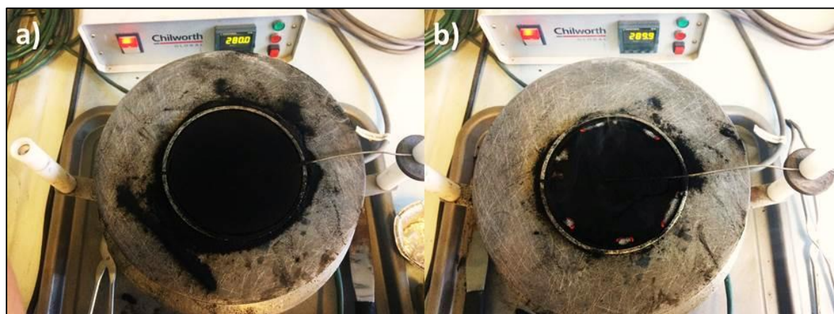
Figure 4.10: Layer of olive pomace dust <250µm in the hot plate test: a) at 280°C not ignition and b) at 290°C ignition.
