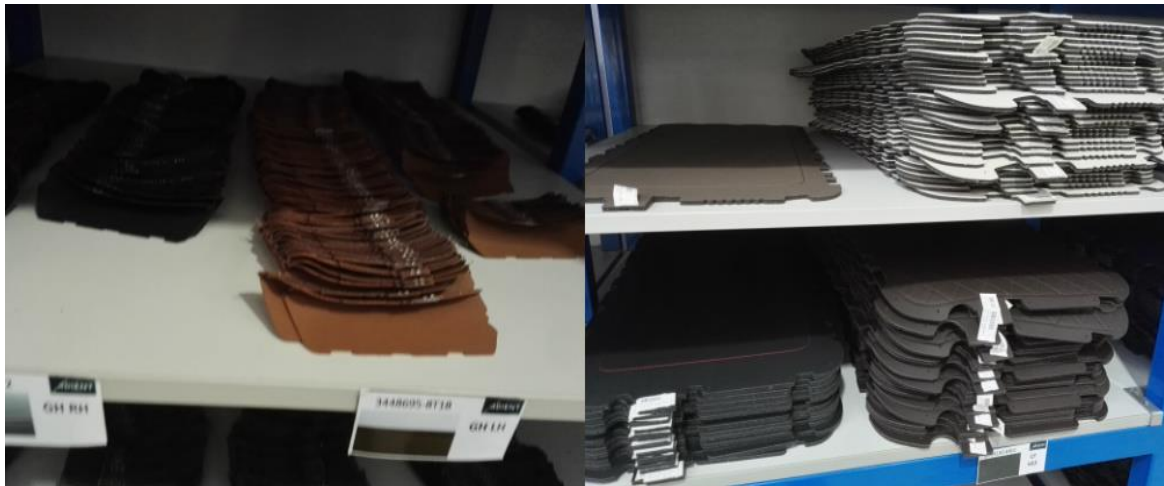
Figure 4.4 Grab handle (on the left) and Centerfield (on the right) leather cover.
