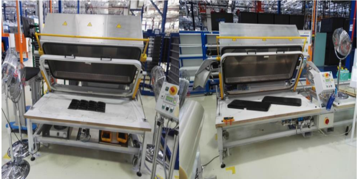
Figure 4.10 Grab handles (on the left) and Centerfield (on the right) vacuum machines.
