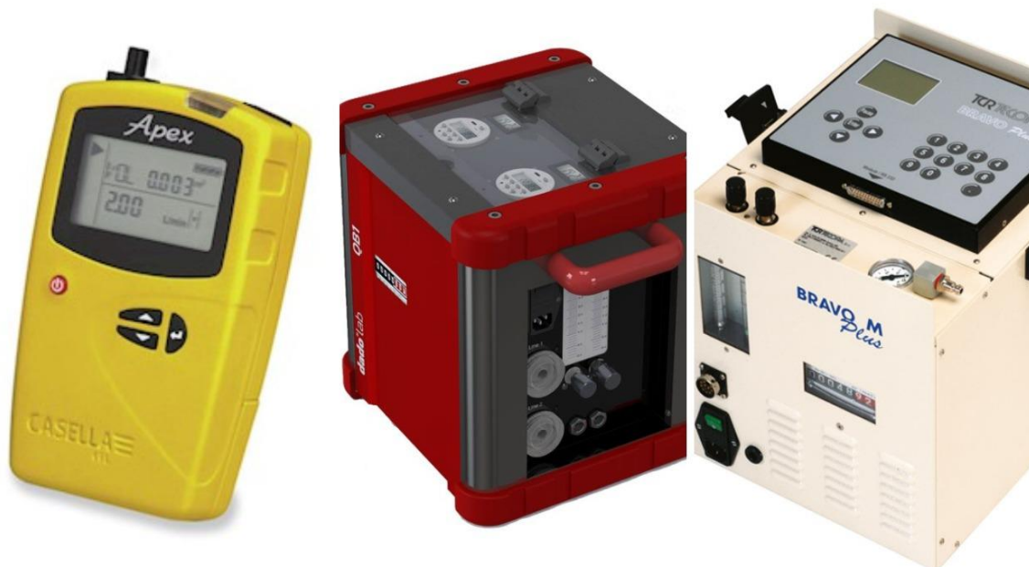
Figure 5.1 The three pumps used for the air measurements in Adient Interiors d.o.o. Kragujevac: digital handheld battery Casella (left), pump for sampling air with constant flow QB1 Dadolab (centre), pump for air sampling Bravo M plus (right).
