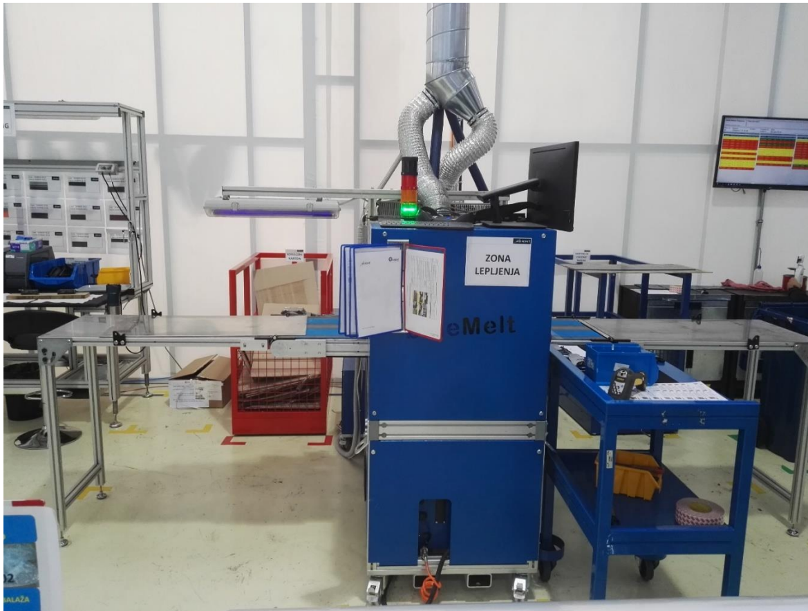
Figure 4.7 Gluing machine in the adhesion zone.
