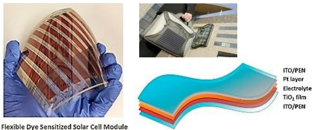
Figure 2.10: Flexible dye-sensitized solar cell printed with the roll-to-roll technology. [40]
