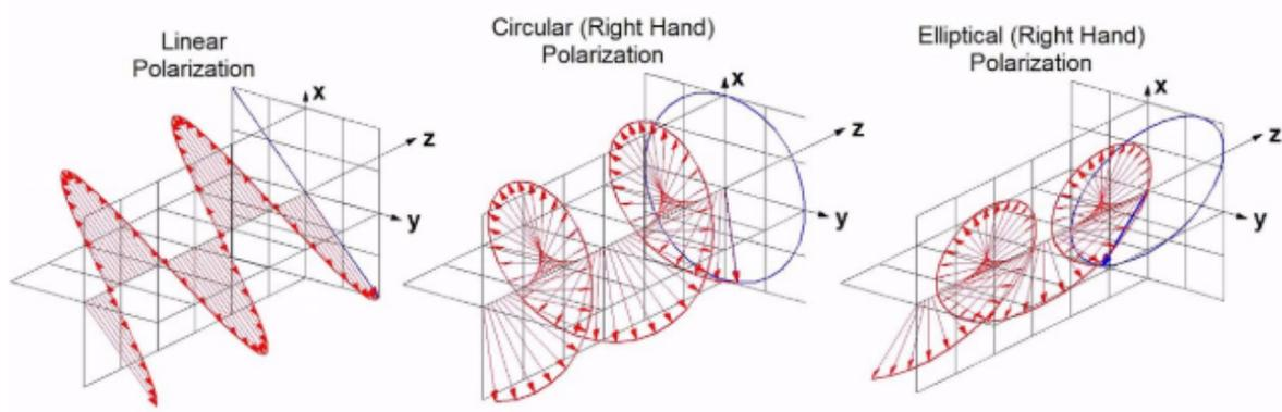
Fig. 3.3 Linear, Circular and Elliptical Polarization
