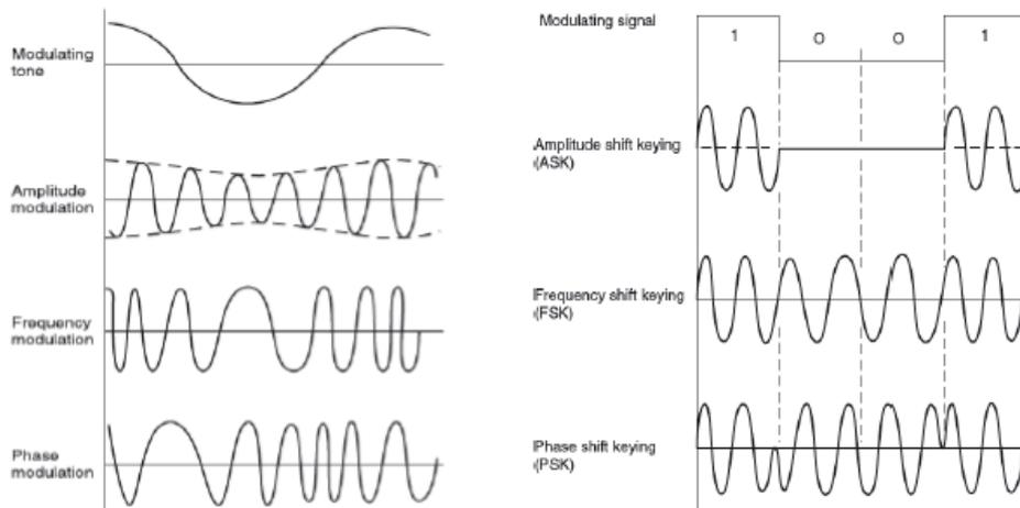
Fig. 3.6 Carrier features that the modulating signal changes
