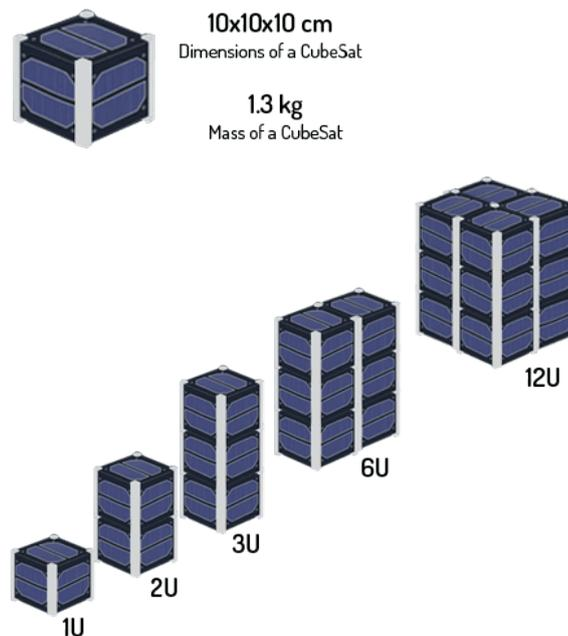
Fig. 1.1 CubeSats dimensions, mass and unit type.
