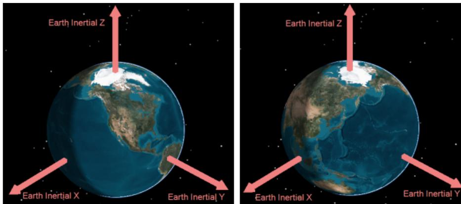
Fig. 4.11 Inertial Reference Frame [3]
