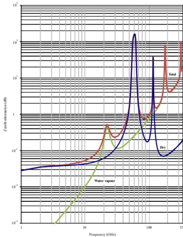
Fig. 3.8 Attenuation of EM Radiation vs. Frequency [8]
