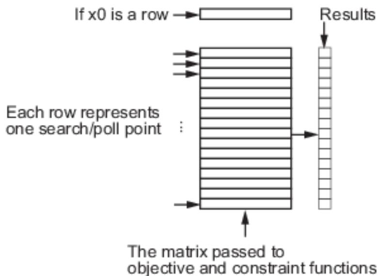
Fig. 4.14 Structure of Vectorized Functions [16]
