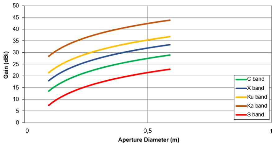
Fig. 3.4 Gain vs. Aperture Diameter for Several Frequencies and aperture Diameters
