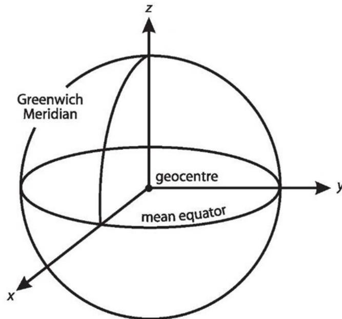
Fig. A.1 Geocentric-equatorial coordinate system
