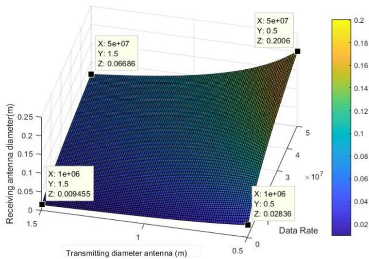
Fig. 3.13 diam r when varying diam t and Data Rate
