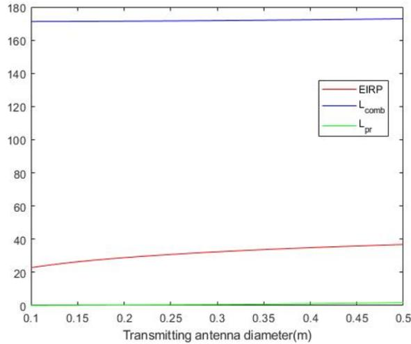
Fig. 3.9 Losses and EIRP when varying diam tx
