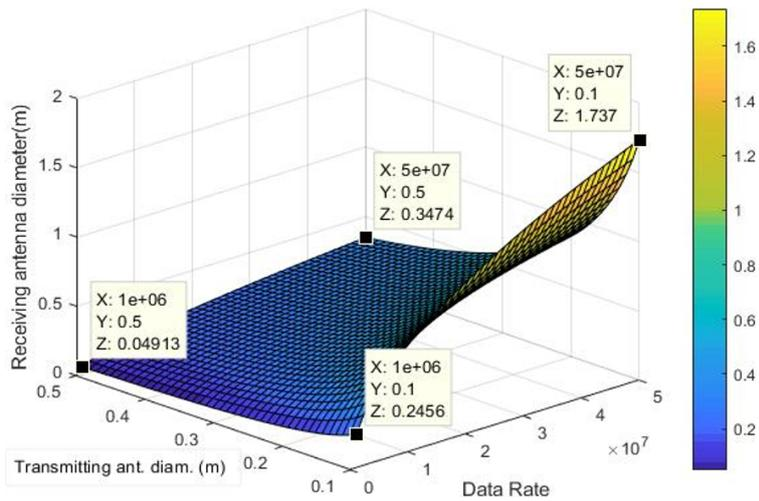
Fig. 3.10 diam r when varying diam t and Data Rate down-link
