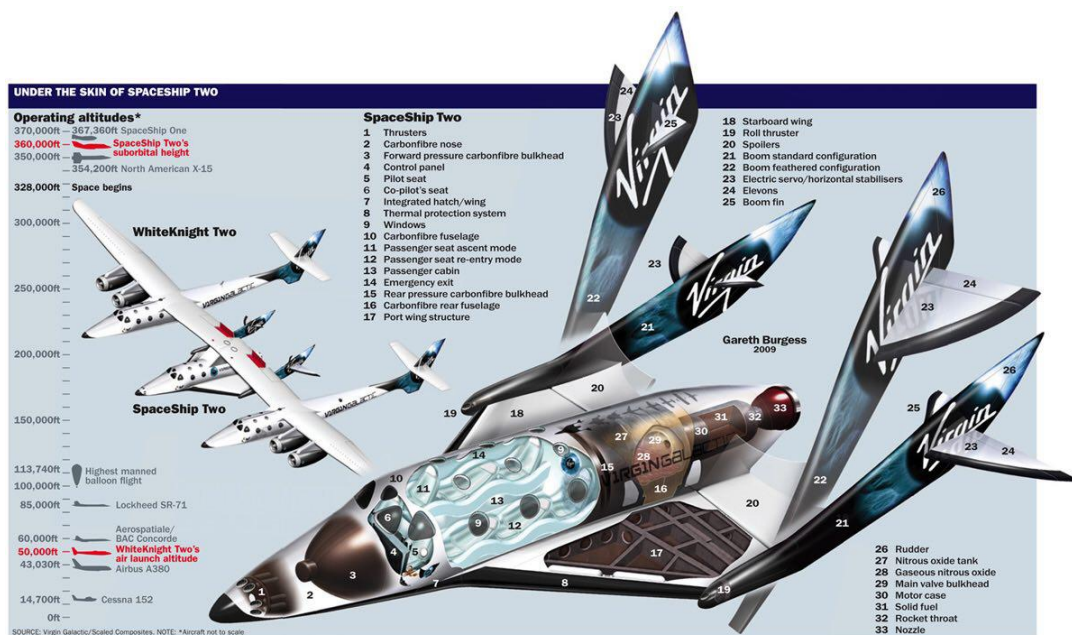
Figure 32: SpaceShipTwo main components [Credits: Virgin Galactic]
