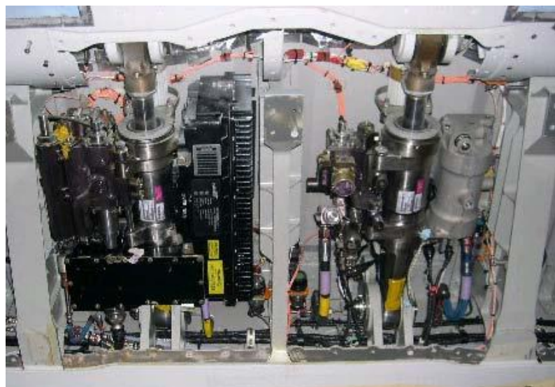
Figure 17: Aileron EHA and electro-hydraulic actuator [23]
