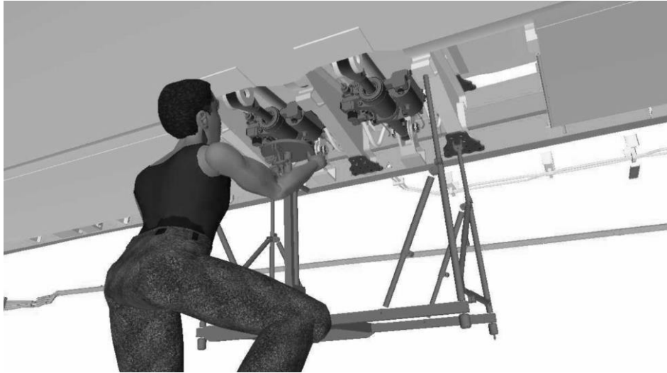
Figure 18: Flight control actuator removal simulation
