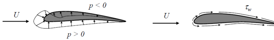
Figure 2.1: Pressure and shear forces acting on body surface
