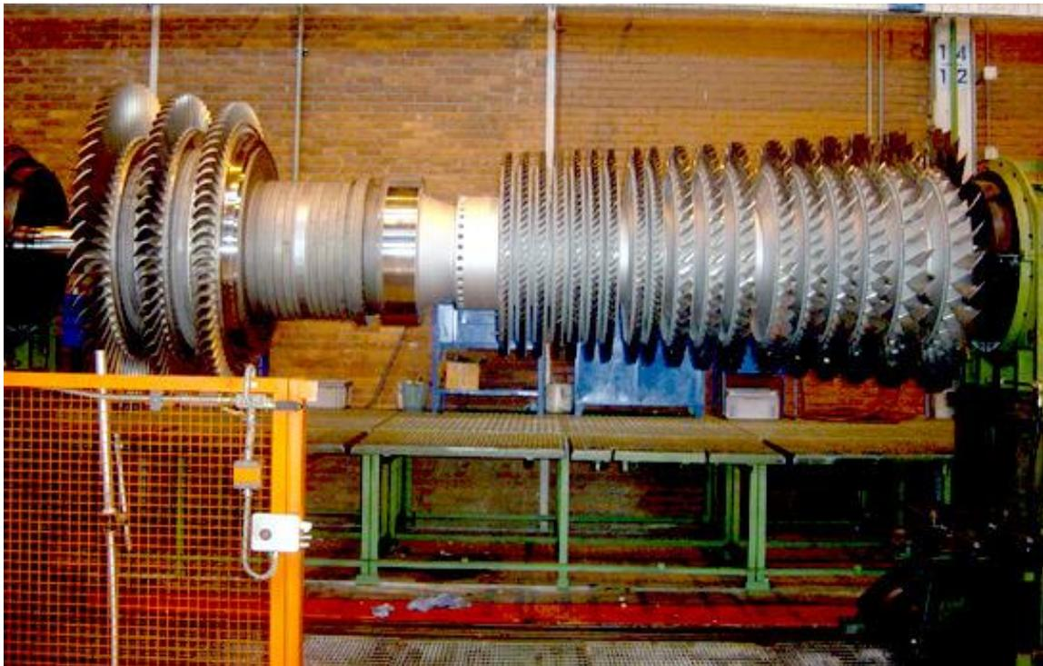
*Figure 1.3: TG20B7/8 turbine, courtesy of EthosEnergy group*
