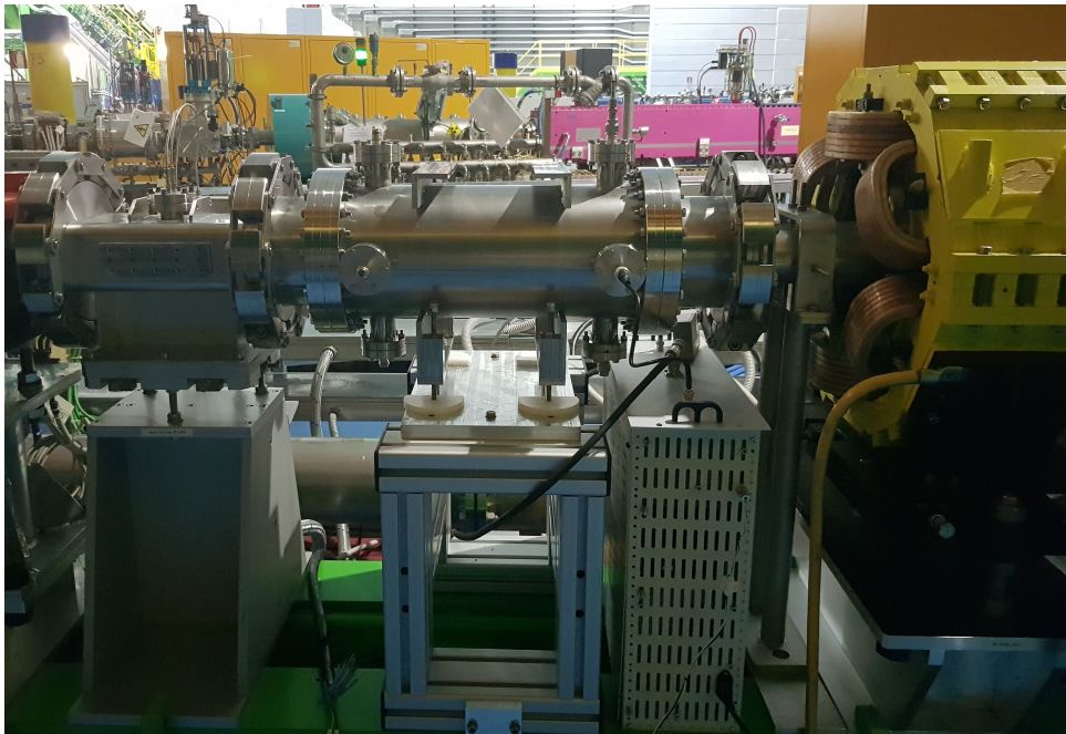
FIGURE 4.12. Picture of the BalUn in the synchrotron room. Observe the cable bringing the signal, the filter and one of the two connections to the kicker's plates.
