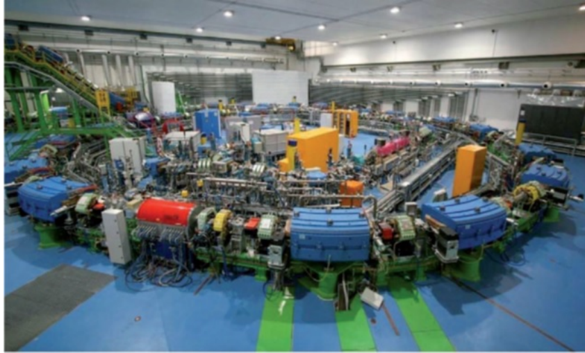
FIGURE 1.11. Real image of CNAO synchrotron. The blue components are the dipoles, while at the centre is possible to observe the LINAC in pink, the electric instrumentation in orange, the sources of hydrogen and bixide carbide in grey. [27].
