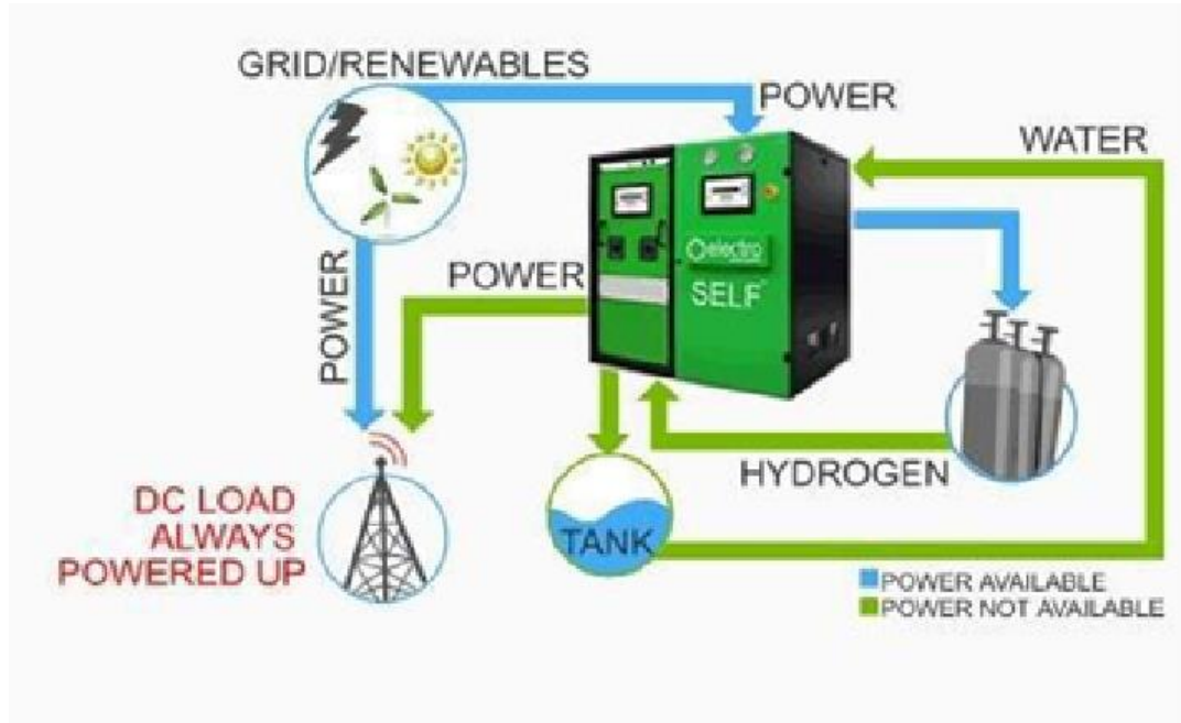
Fig. 1.2.1: electrolyzer operating scheme.
