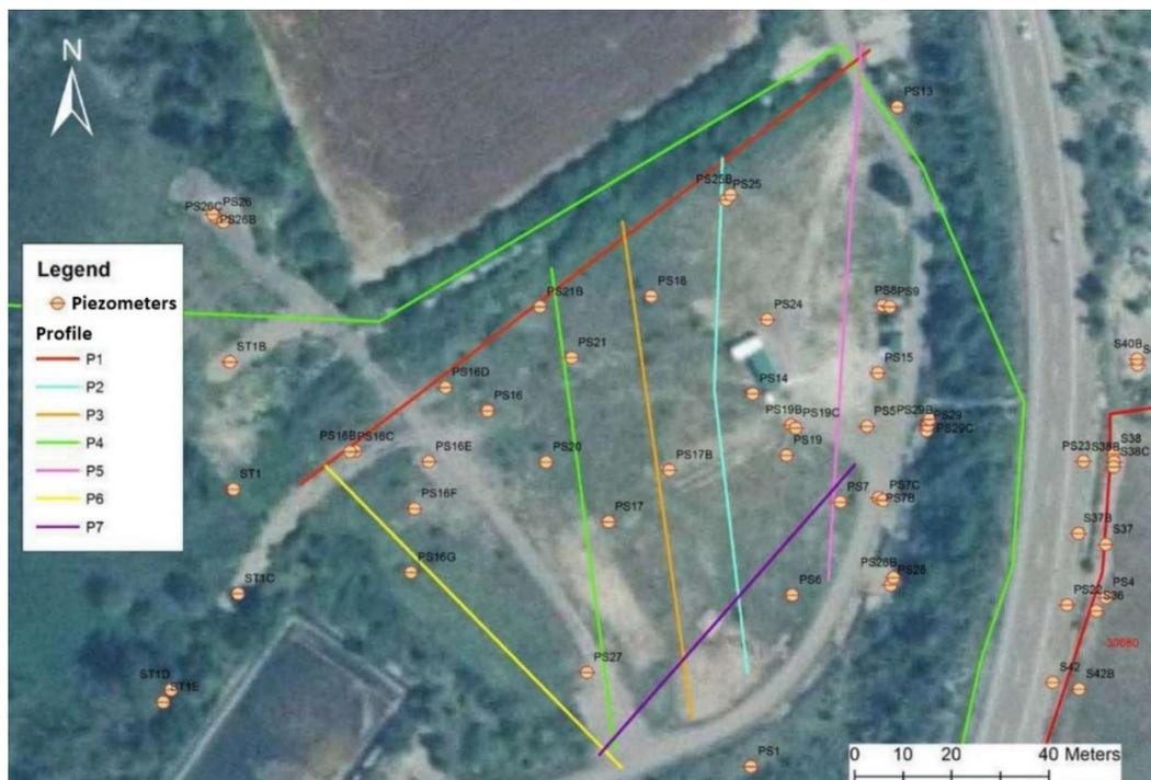
Figure 13: profiles used in the electric tomography test
