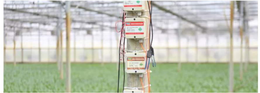
Plant body sensing sensor monitors plant growth process in real time
