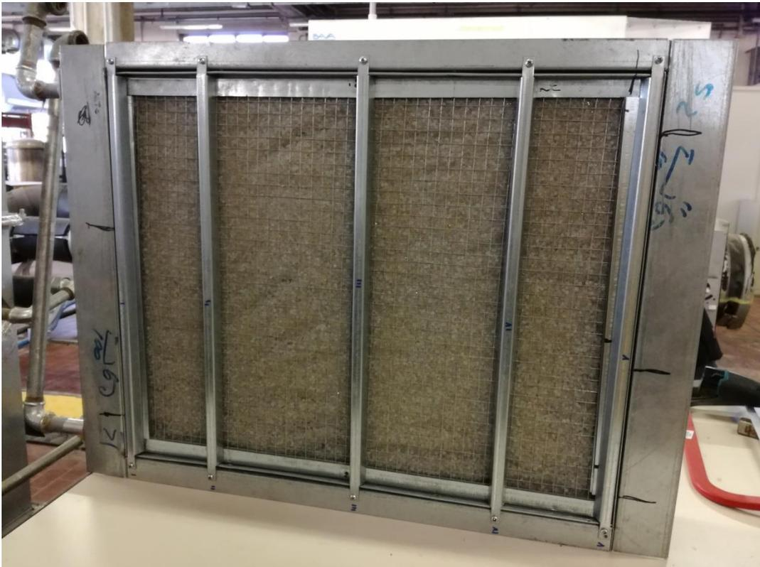
**Figure 31 – Silica gel battery**
