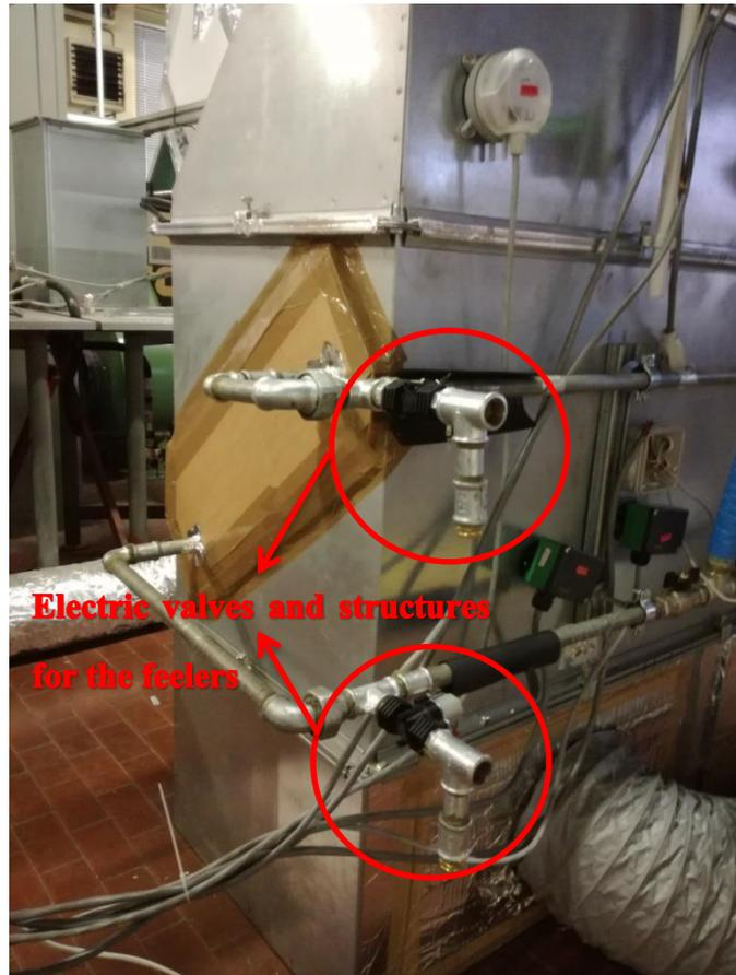
**Figure 36 – Cooling connections**
