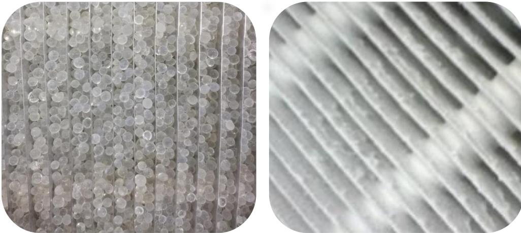
**Figure 33 – Particular of the adsorbent material. On the left silica gel while on the right zeolite**
