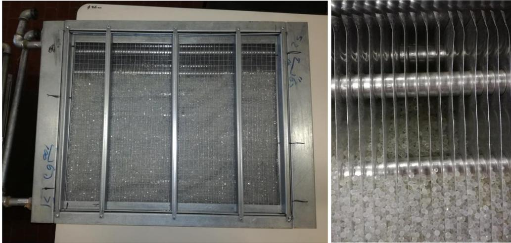
**Figure 34 – Banking of silica gel grains**
