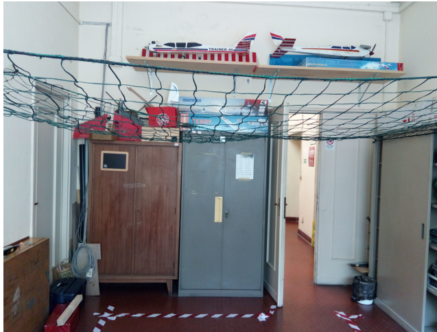
Figure 4.16: A net is used as the reference plane for Px4flow
