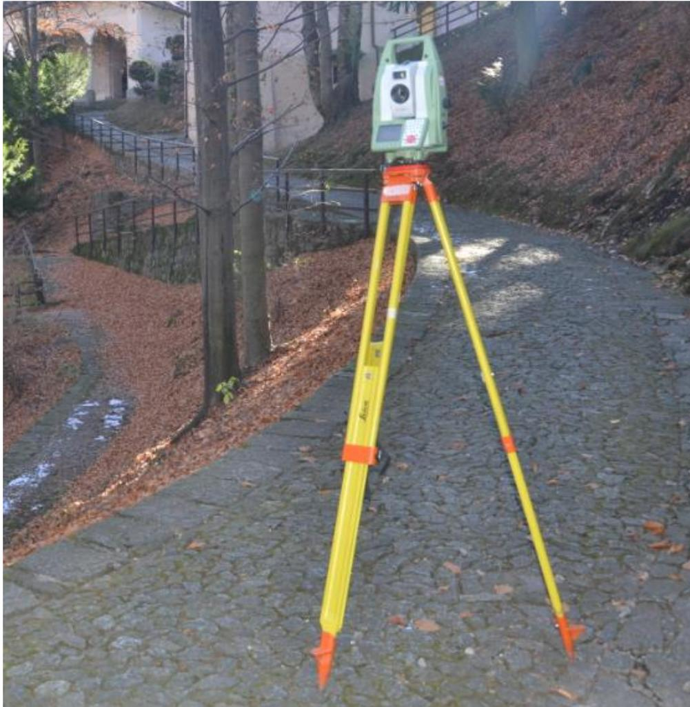
*Figura 24 - Leica Nova Scan Station
