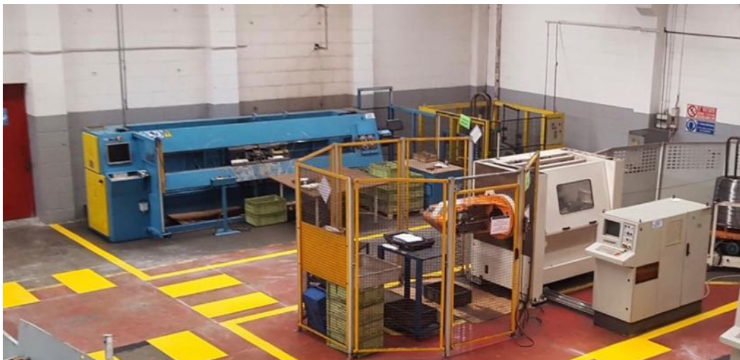
Figure 19 Bending work cell
