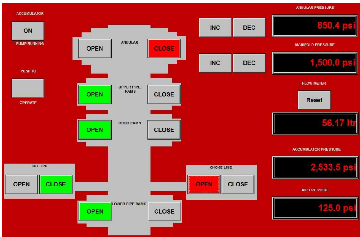
Figure 5- Shut in the well from BOP
