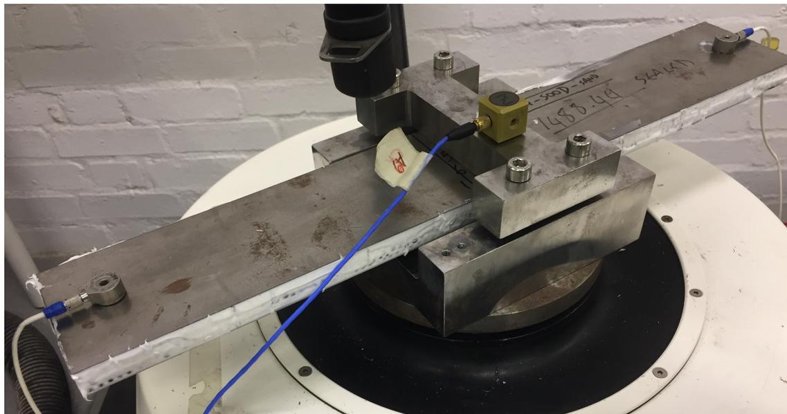
Figure 6.3: The specimen with a PCB piezoelectric accelerometer.
