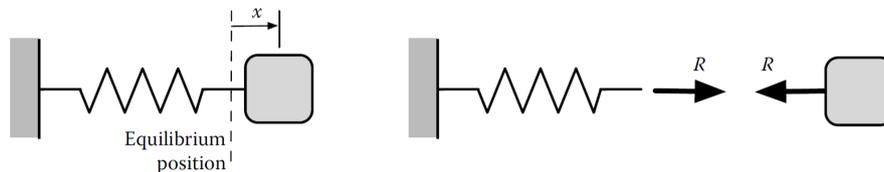
Figure 4.1: Displacements and forces in a simple mass-spring system [19].
