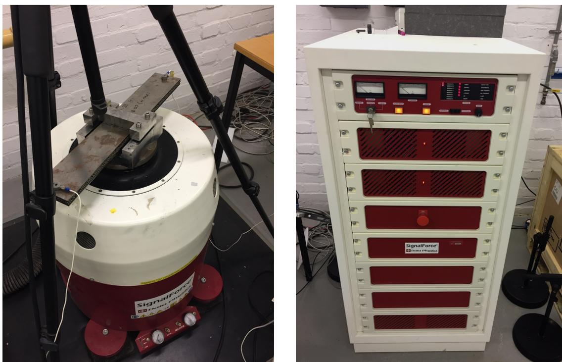
Figure 6.2: Electrodynamic Shaker V400HG/DSA4 of Data-Physics
