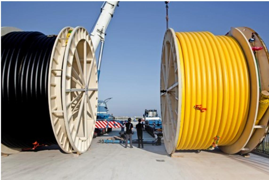
Figure 3.5: Massive spools of Airborne Oil and Gas' thermoplastic composite pipe.
