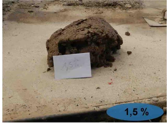
*img. 2 – Mixture of clay and waste textile in polyester, with concentration of 1,5%.*
