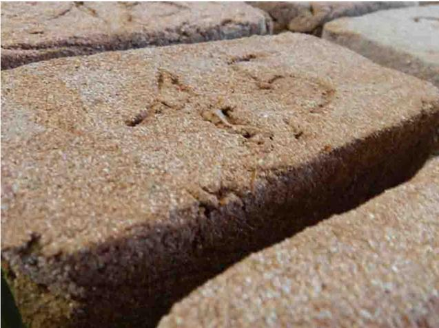
*img. 3 – Sample of experimental brick MAST with dimensions of 120x60x30mm.*
