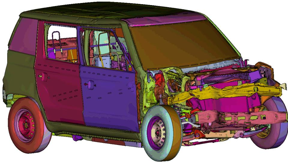
Figure 5.71: U Model MPDB - structural collapse detail
