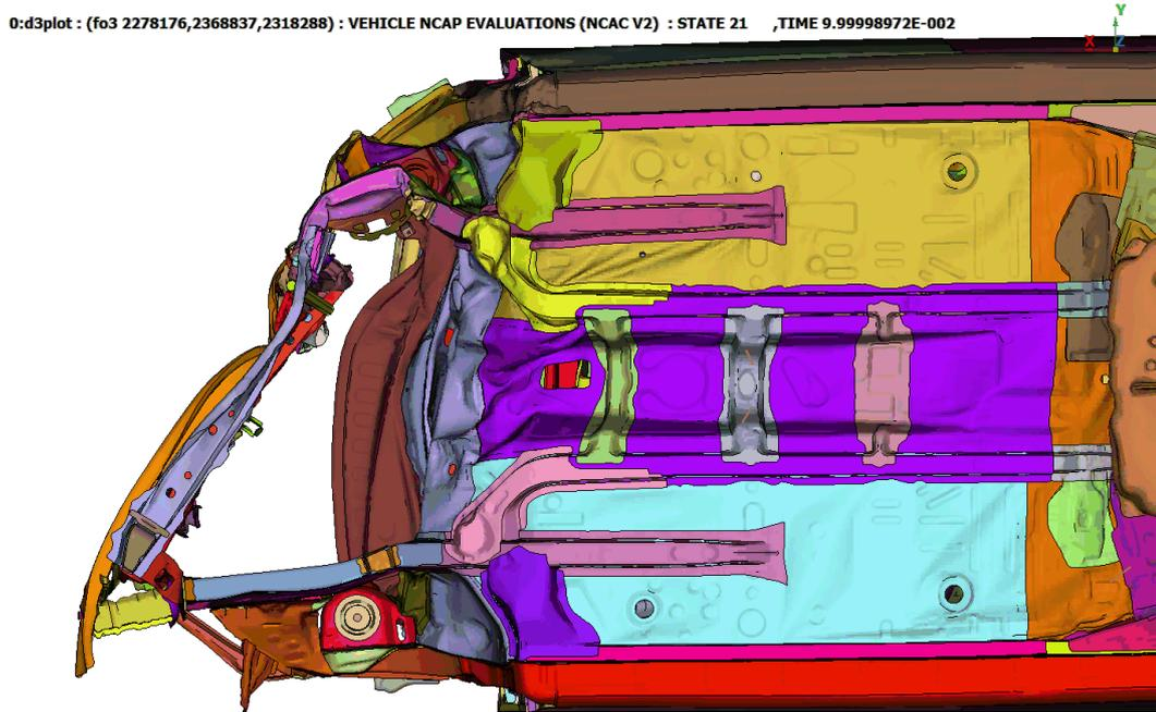
Figure 5.2: Toyota Yaris ODB - structural collapse detail
