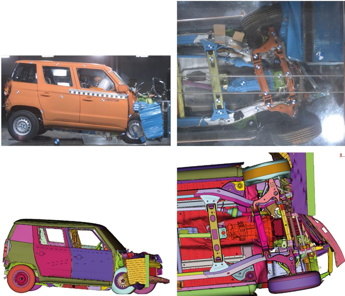
Figure 4.25: U Model ODB 56km/h - RHS and underbody comparison
