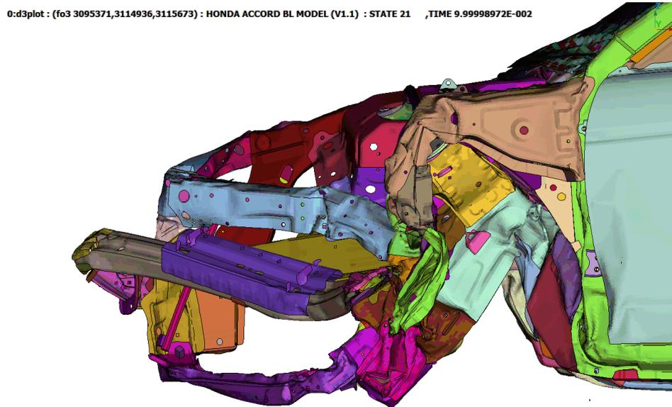
Figure 5.35: Honda Accord MPDB - structural collapse detail
