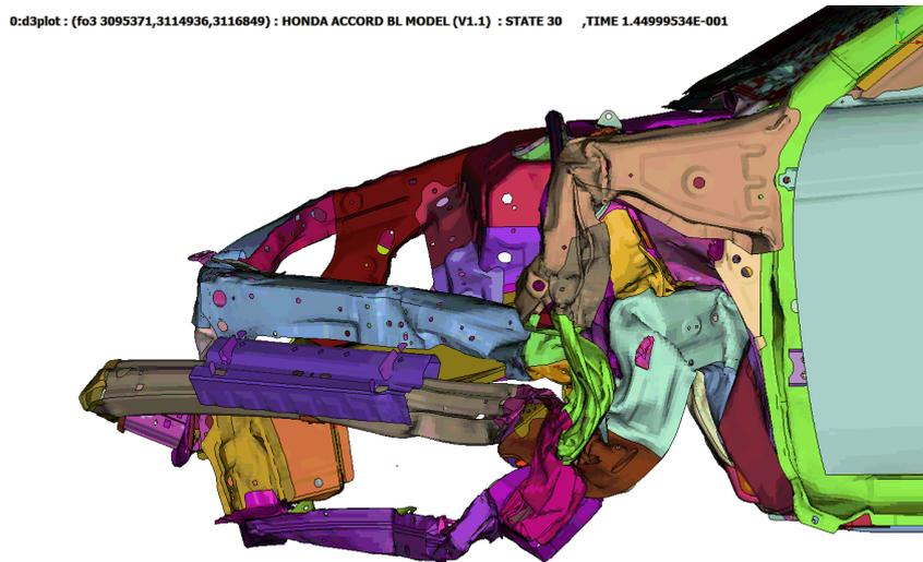
Figure 5.31: Honda Accord ODB - structural collapse detail
