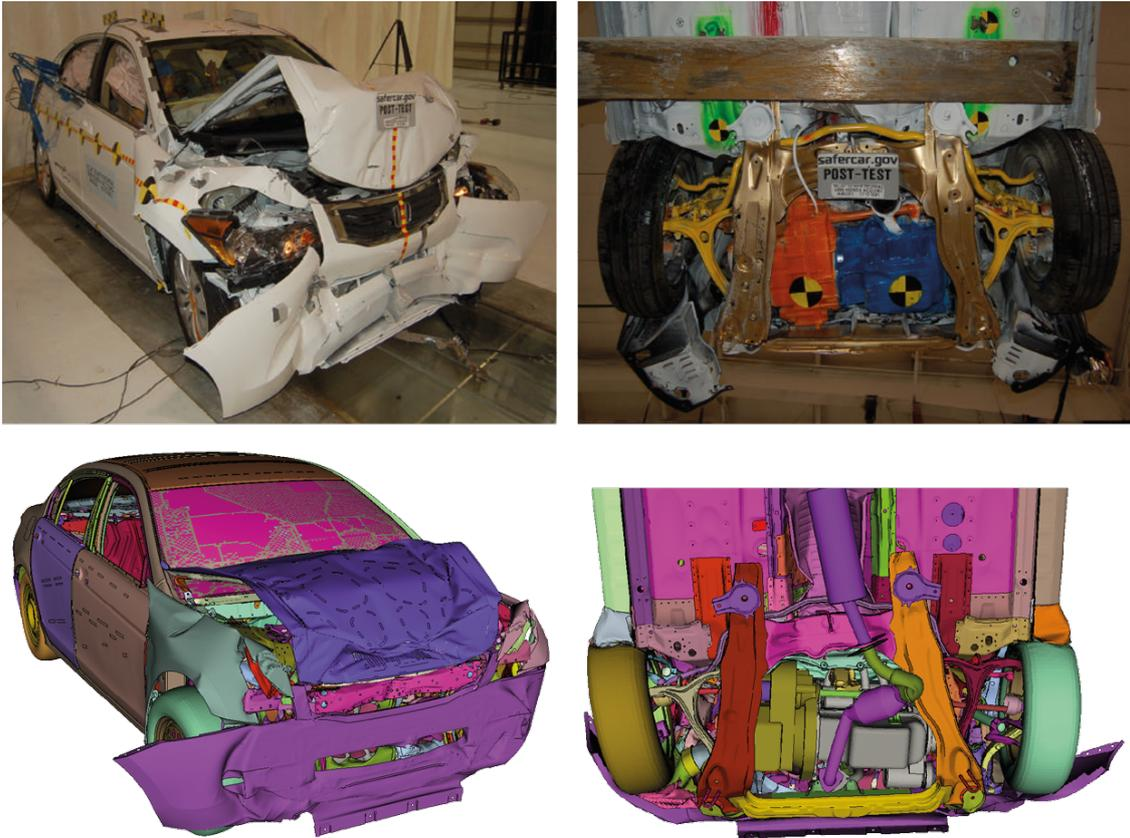
Figure 4.16: Accord FWRB - three quarters and underbody comparison
