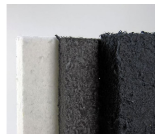
Example of sound materials; porous absorbing material (cotton) (Adams, 2016)
