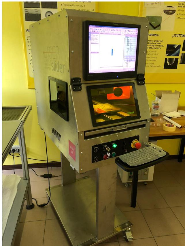
Figure 3.1: Laser  $CO_2$  present in Microla Optoelectronics laboratory in Chivasso
