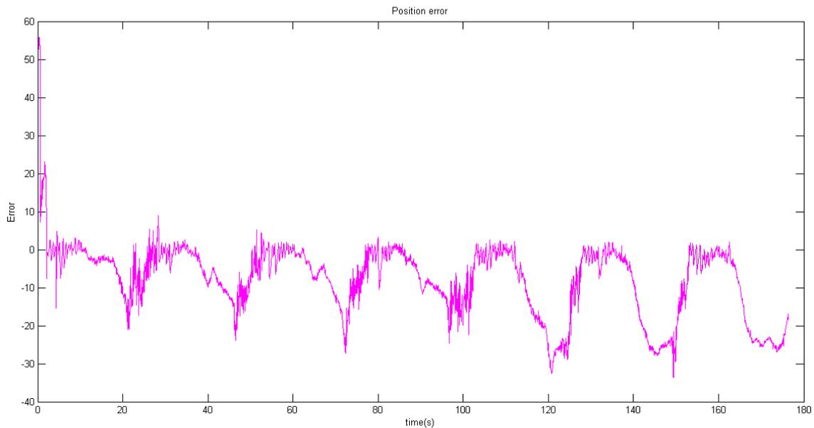
Figure 4.9: System error in extension for sinusoidal input.
