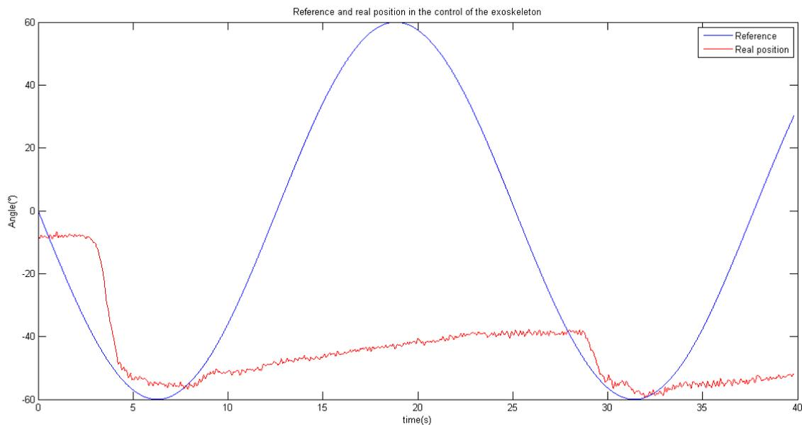
Figure 4.13: System response in flexion for a sinusoidal input.
