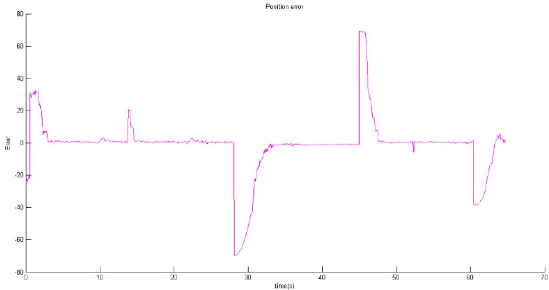
Figure 4.18: System error in flexion-extension for a step input.
