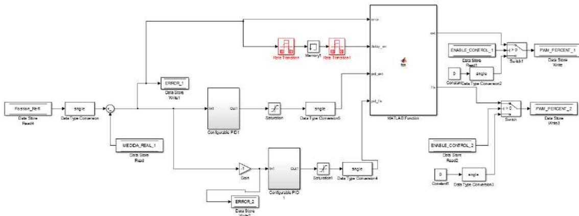
Figure 3.20: Control system for 2 actuators.
