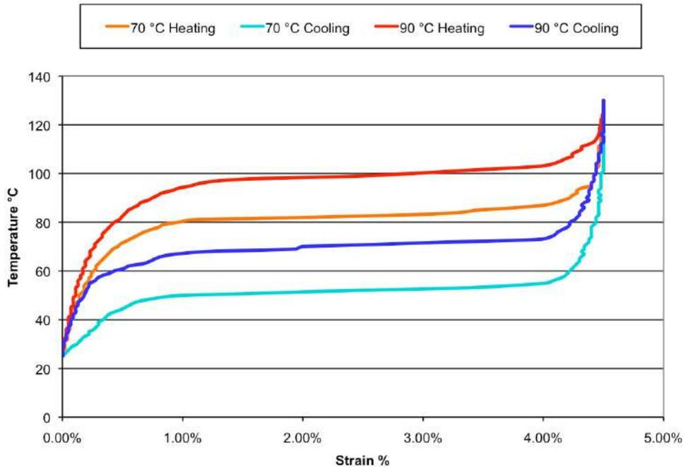
Figure 3.16: SMA strain percentage with the temperature [Appendix A].
