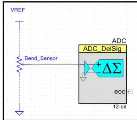
In this configuration the voltage that the ADC will measure will increase or decrease depending on the direction the Bend Sensor<sup>®</sup> is bent. Because each individual Bend Sensor<sup>®</sup> cannot go to zero ohms of resistance the response curve looks similar to a hyperbolic tangent function:
