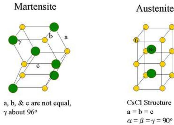
Figure 2.13: Martensite and austenite microstructure of Nitinol.
