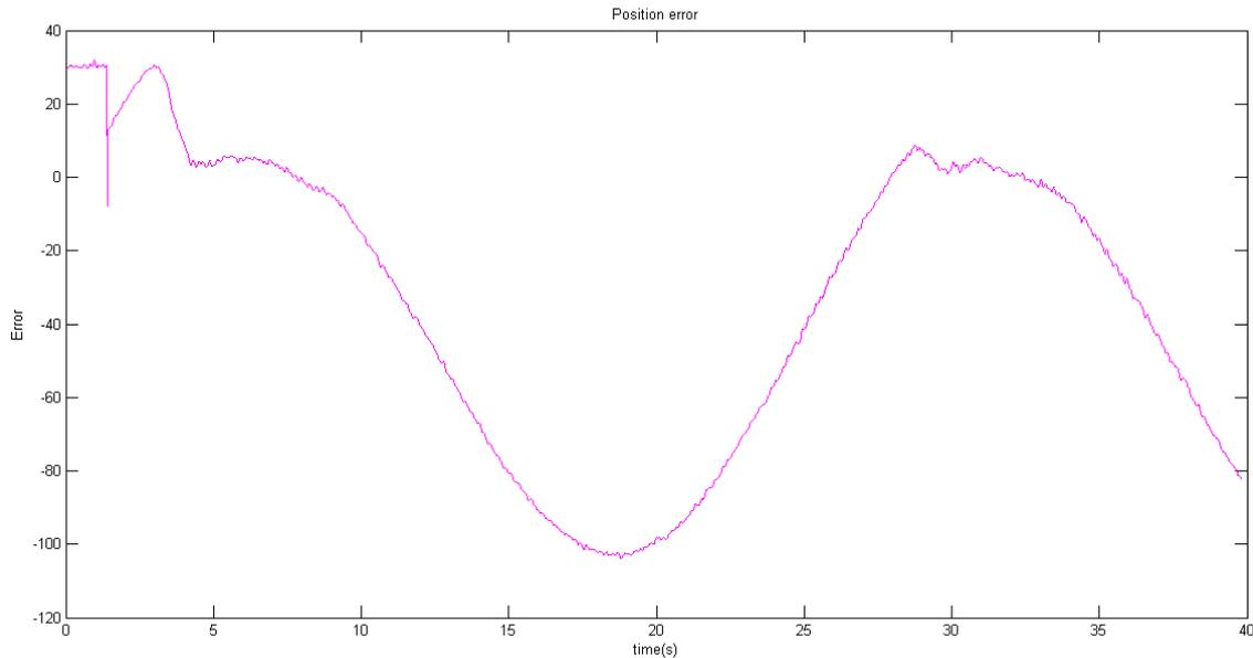
Figure 4.15: System error in flexion for a sinusoidal input.
