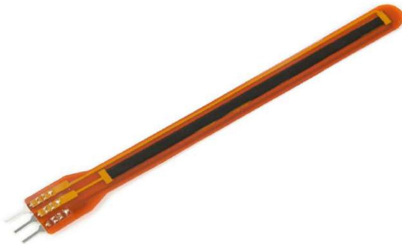
Figure 3.13: Bi-directional bend sensor.
