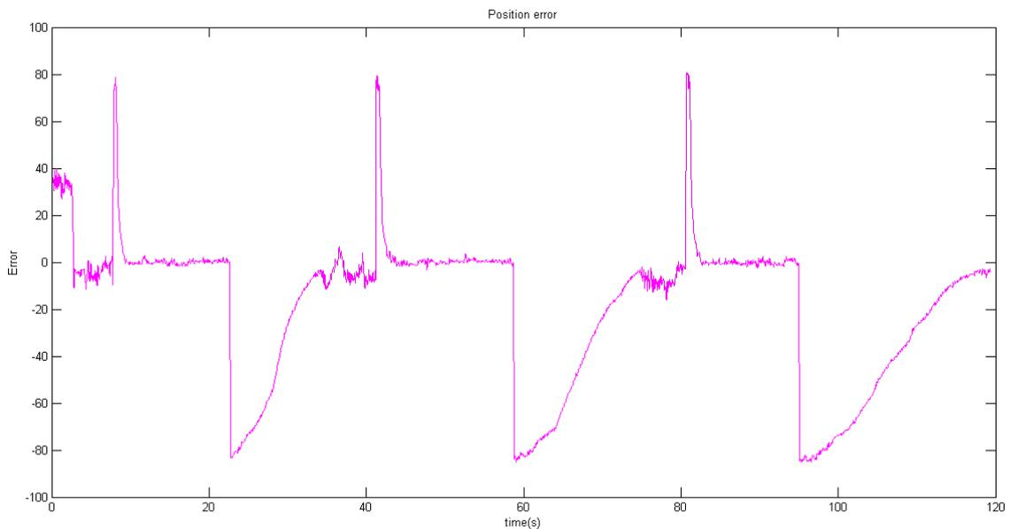
Figure 4.3: System error in extension for step input.
