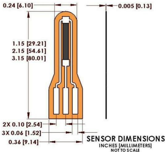
The stock product BEND SENSORS® are available in 1", 2" and 3" lengths. Custom sensor designs can be produced to meet customer requirements.
