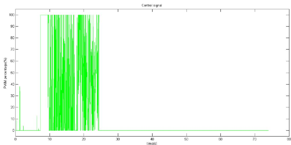
Figure 4.11: Control signal in flexion for a step input.
