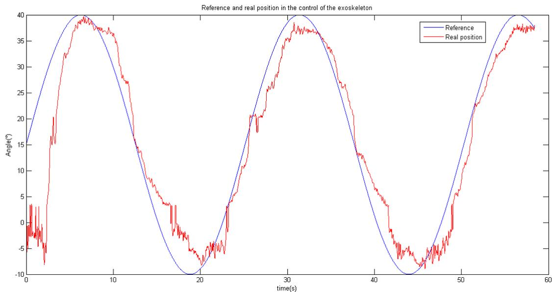
Figure 4.31: System response in ulnar-radial deviation for a sinusoidal input.
