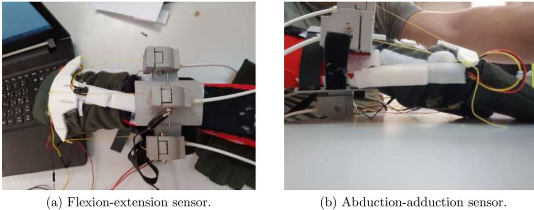
Figure 3.14: Position of the sensors.
