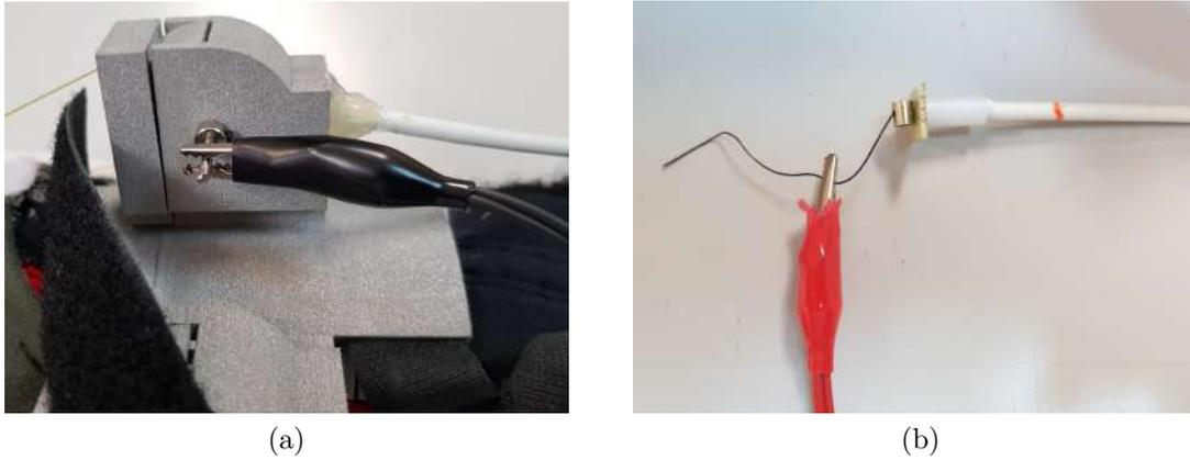
Figure 3.23: Connection of the SMA actuator to the electronic circuit.
