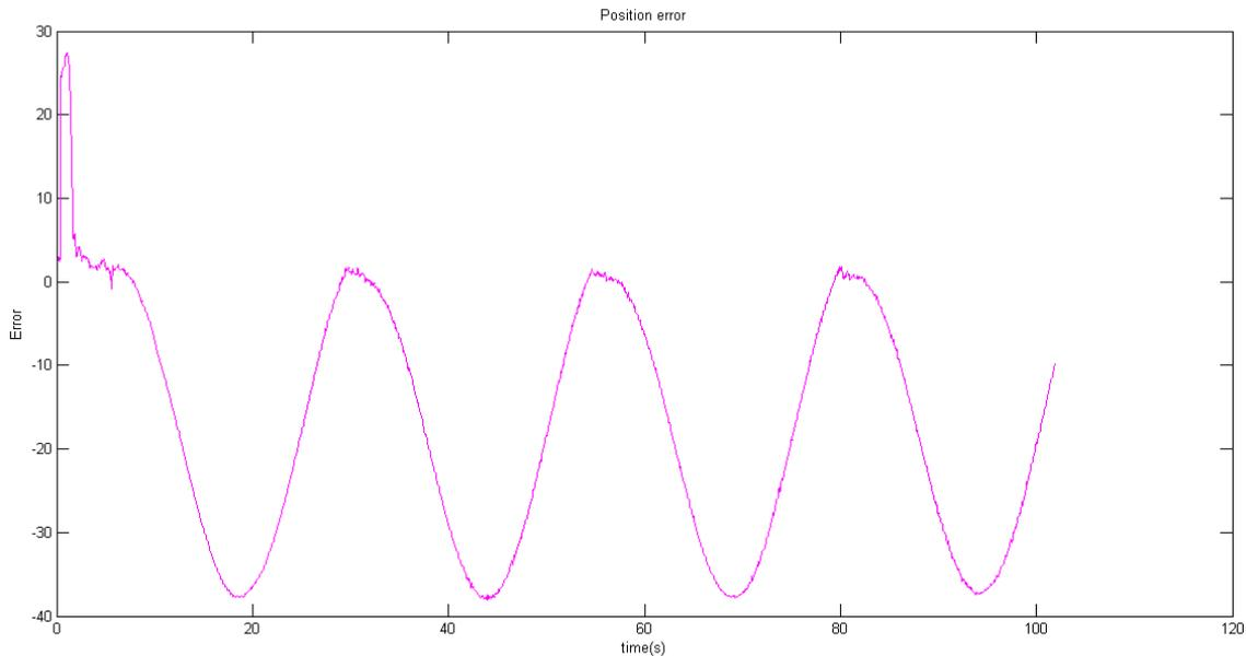
Figure 4.24: System error in ulnar deviation for a sinusoidal input.
