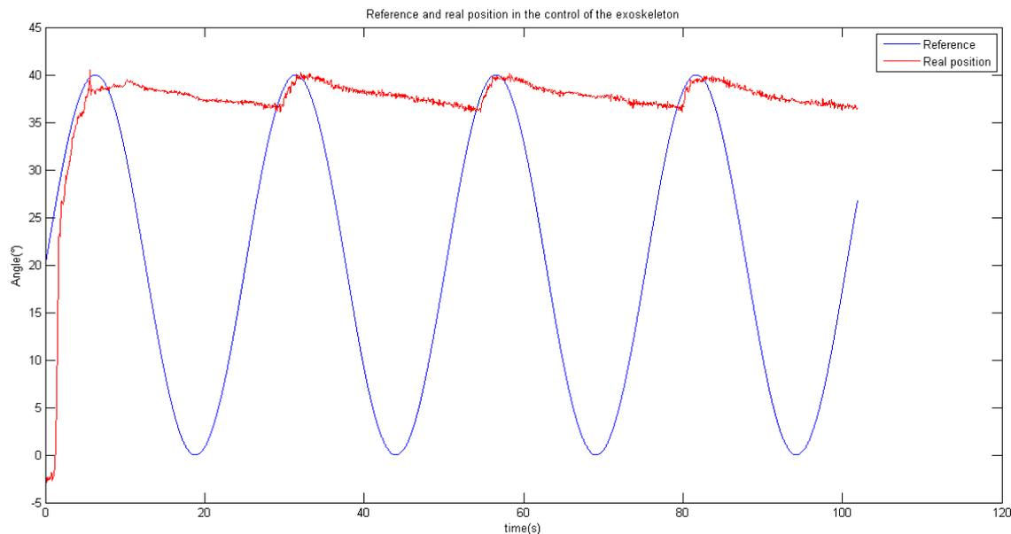
Figure 4.22: System response in ulnar deviation for a sinusoidal input.
