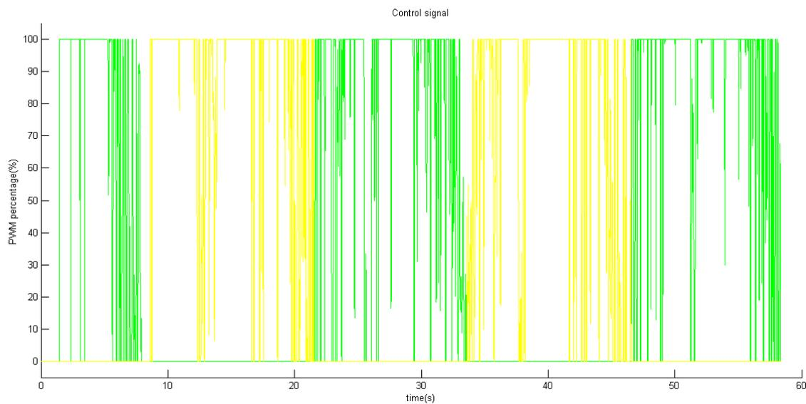
Figure 4.32: Control signal in ulnar-radial deviation for a sinusoidal input.
