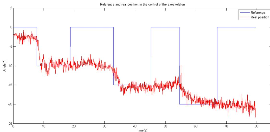
Figure 4.25: System response in radial deviation for a stair input.
