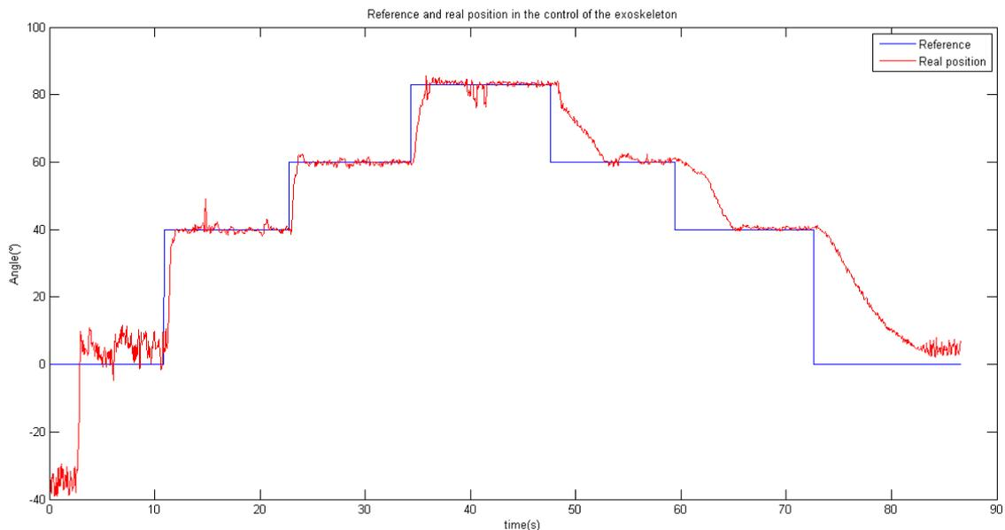
Figure 4.4: System response in extension for stair input.
