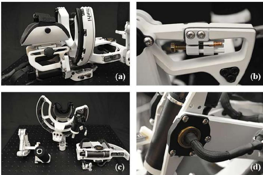
Figure 2.11: OpenWrist Features – (a) central hub with curvilinear rails, (b) integrated quick connect tensioner, (c) modular assembly allows for ambidextrous configurations, (d) electrical wire routing through joint axes[6].
