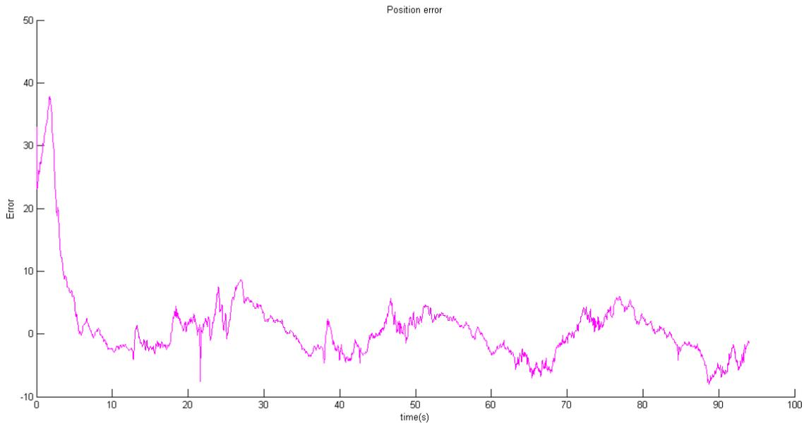
Figure 4.21: System error in flexion-extension for a sinusoidal input.
