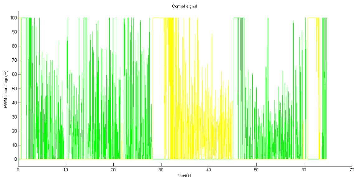
Figure 4.17: Control signals in flexion-extension for a stair input.
