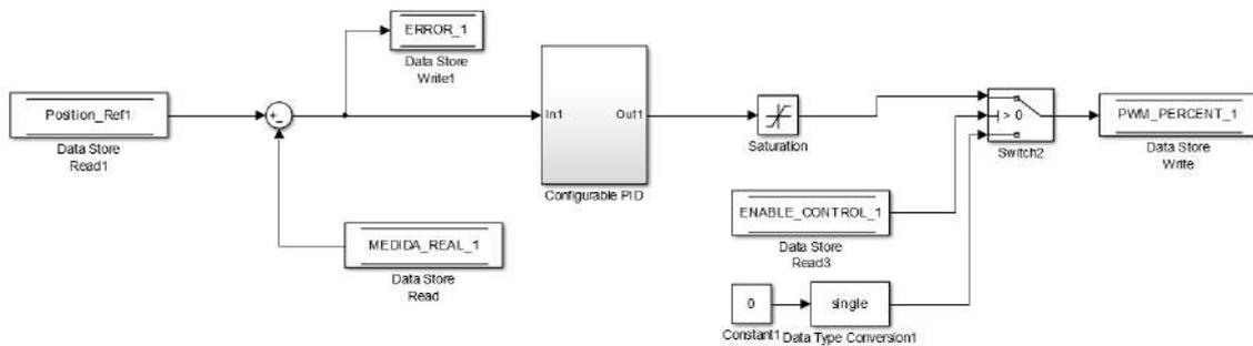
Figure 3.19: SMA control loop.
