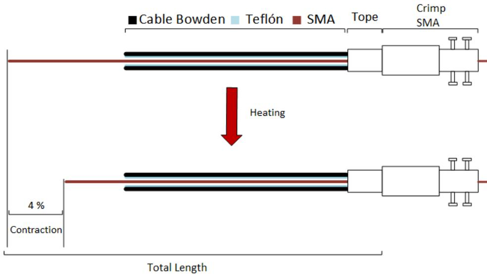
Figure 2.16: SMA actuator design.
