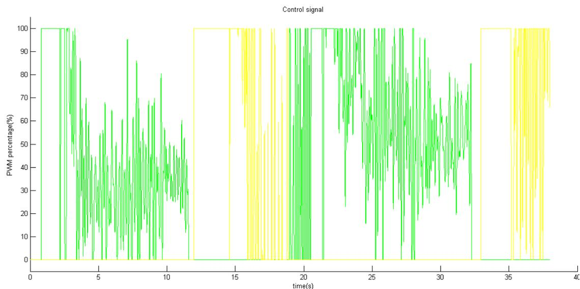
Figure 4.29: Control signal in ulnar-radial deviation for a stair input.
