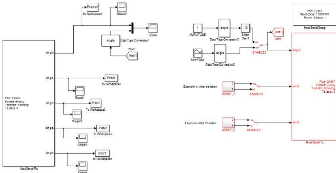
Figure 3.21: Host block scheme to control the exoskeleton.
