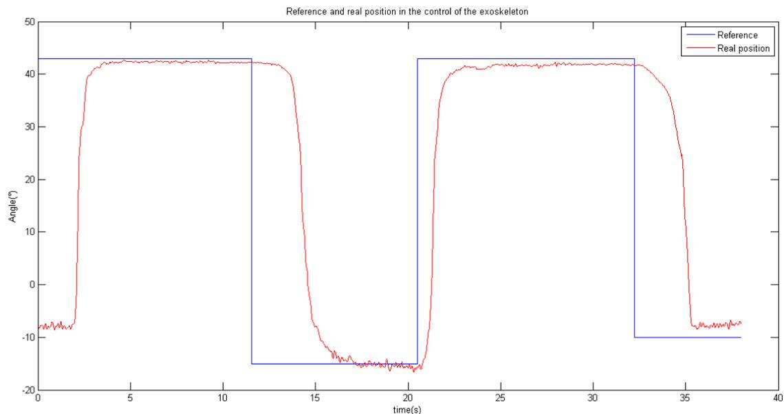
Figure 4.28: System response in ulnar-radial deviation for a stair input.
