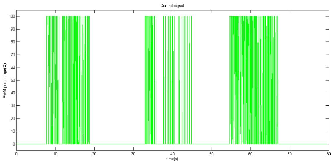
Figure 4.26: Control signal in radial deviation for a stair input.
