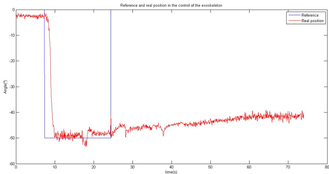
Figure 4.10: System response in flexion for a step input.
