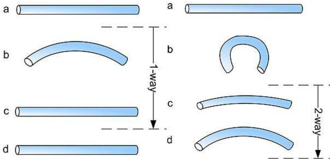
Figure 2.15: 1-way and 2-way shape-memory effects.
