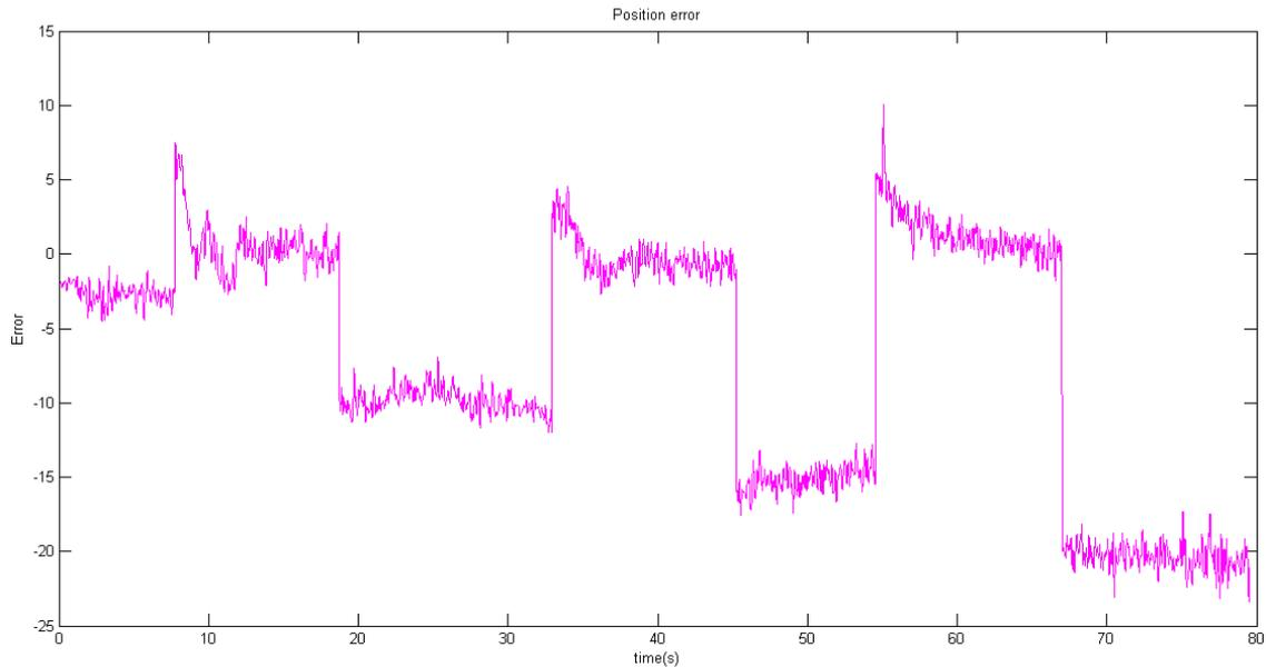
Figure 4.27: System error in radial deviation for a stair input.
