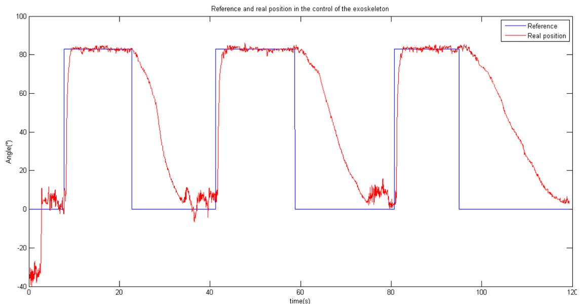
Figure 4.1: System response in extension for step input.
