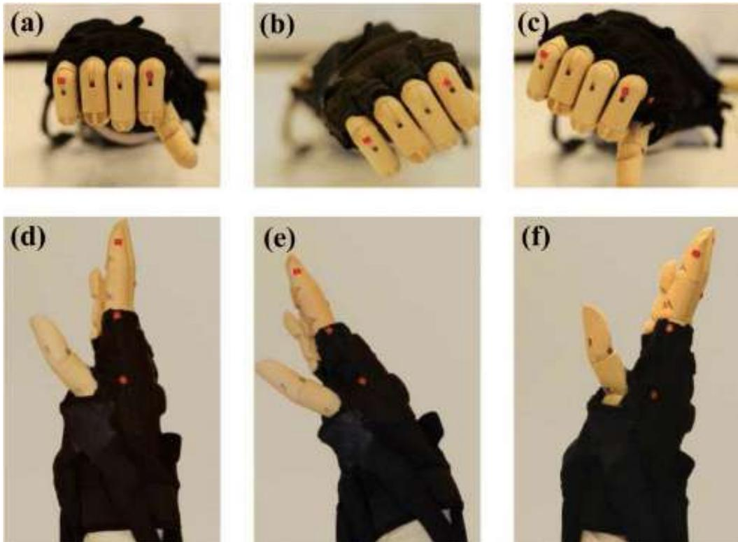
Figure 2.9: (a)Device off, (b)supination, (c)pronation, (d)device off, (e)flexion, and (f)extension [4].
