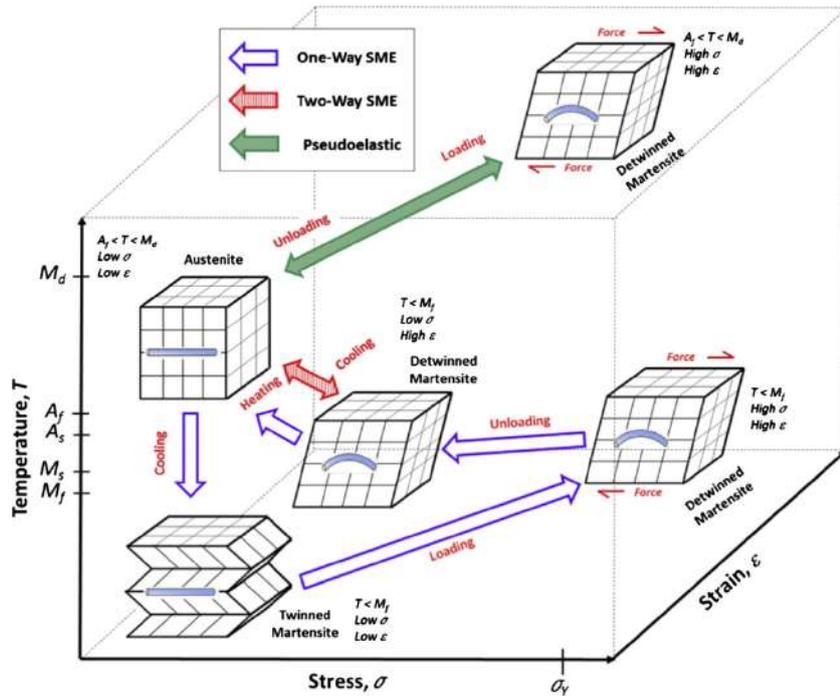
Figure 2.12: SMA phases and crystal structures [7].
