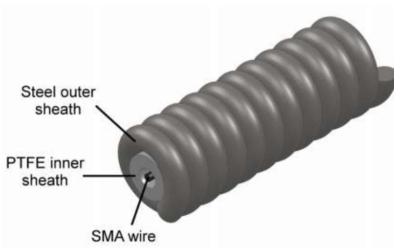
Figure 2.17: CAD model showing the actuator configuration [19].
