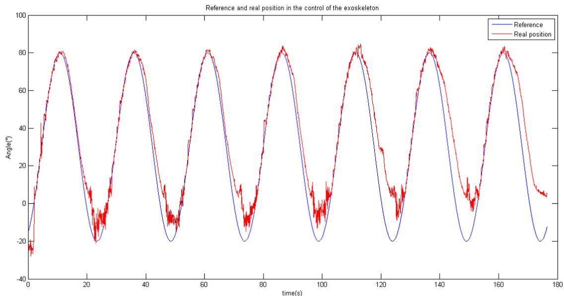
Figure 4.7: System response in extension for sinusoidal input.
