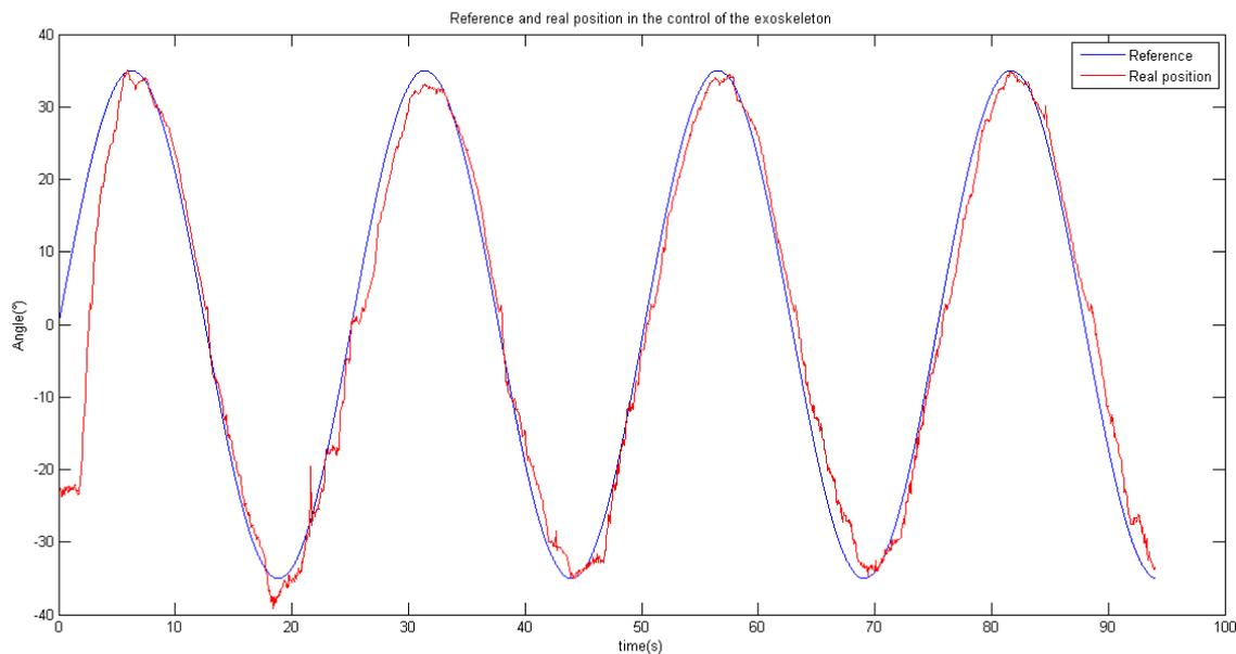
Figure 4.19: System response in flexion-extension for a sinusoidal input.
