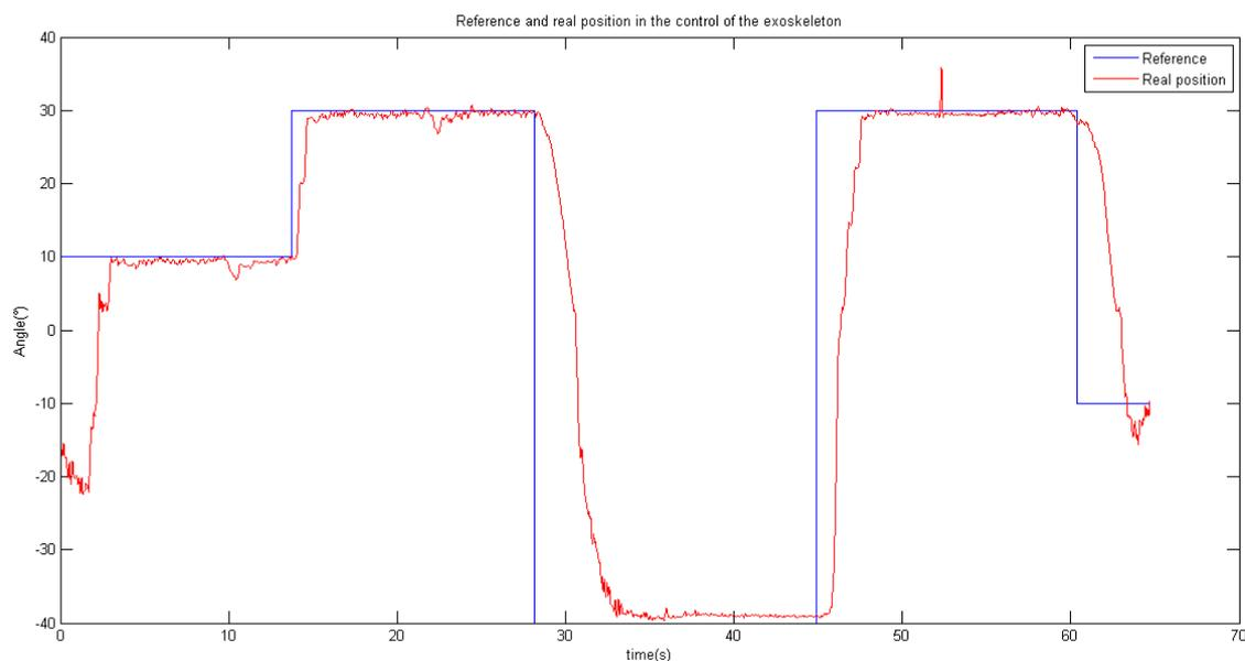
Figure 4.16: System response in flexion-extension for a stair input.
