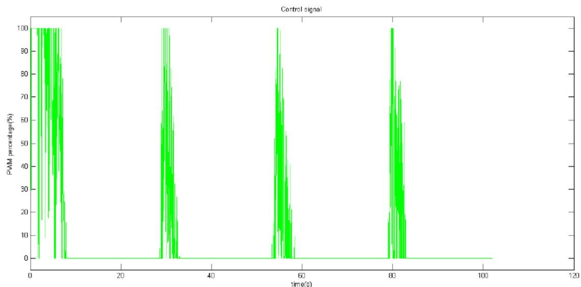
Figure 4.23: Control signal in ulnar deviation for a sinusoidal input.
