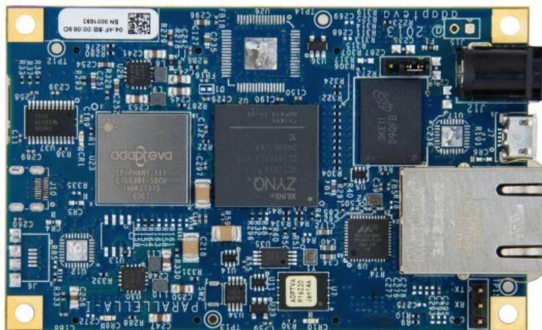
Figure 3.1. The Parallella board
