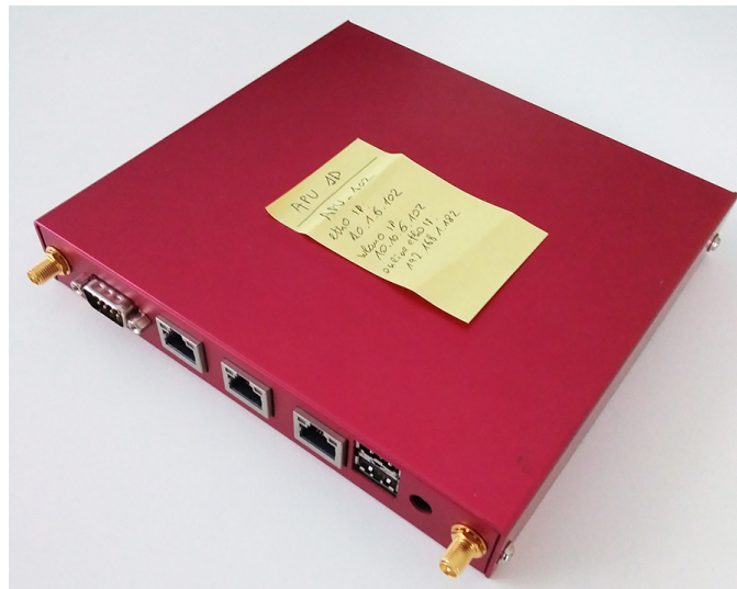
Figure 5.1: ALIX 1d board view from outside, with the UNEX card and the enclosure mounted on. It is possible to distinguish the DB9 serial connector, the three Ethernet ports, two USB ports and the DC power connector, together with two RP-SMA connectors for two antennas.
