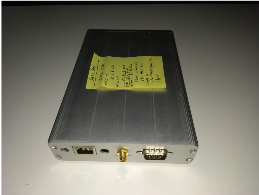
Figure 3.1: ALIX 3d2 board view from outside, with the enclosure mounted on. It is possible to distinguish the Ethernet port, the DB9 serial connector, a 50 \omega impedance RP-SMA connector connected to the wireless card and the DC power connector.
