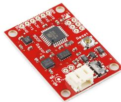
**Figure 2.8:** 9DOF Razor IMU sensor
