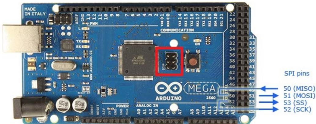
**Figure 4.5:** Arduino Mega 2560 SPI pins
