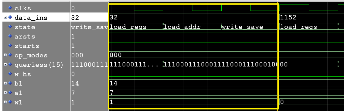
Figure 4.6: Waveform of a Write operation
