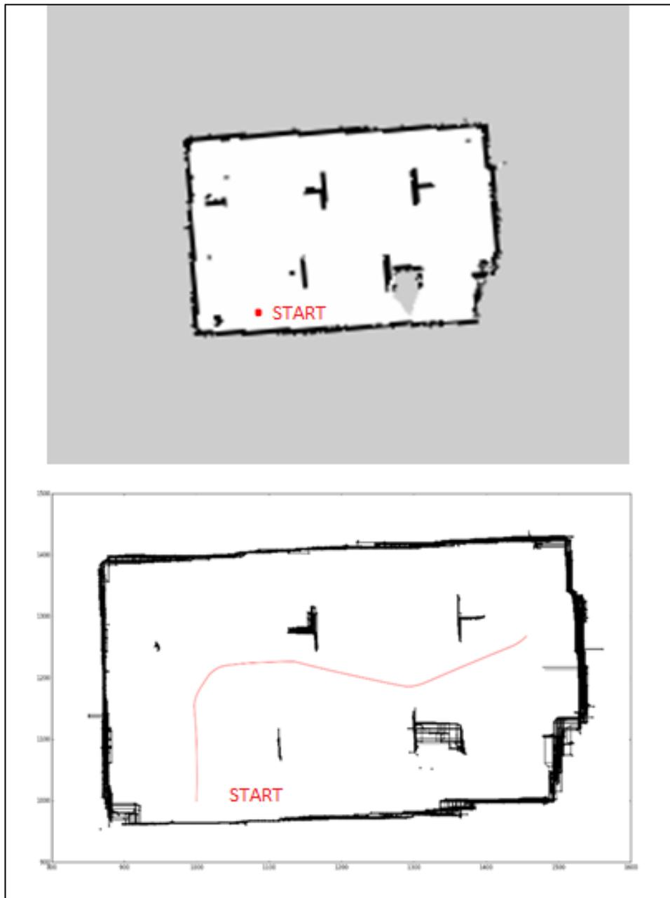
*Figure 5.8: a) LIM room map realized by Gmapping at 2 Hz
