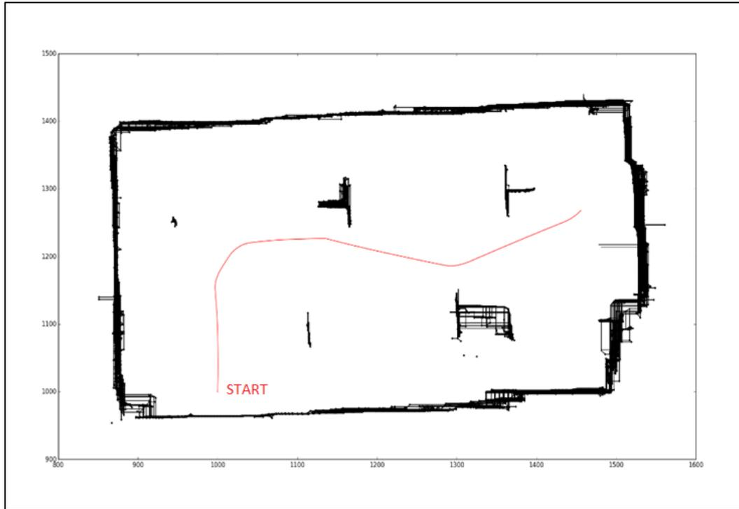
*Figure 5.5: LIM room map realized by OccGridMapp with Optimization*
