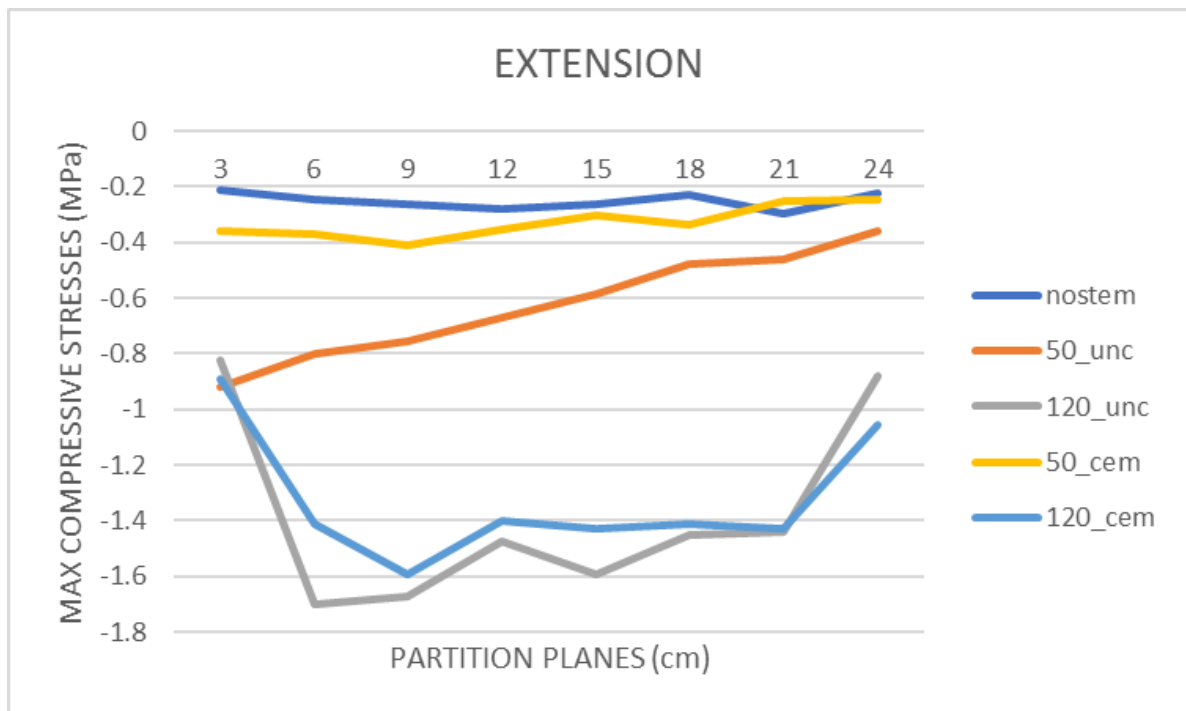
Fig.56 Maximum Compressive Stresses for the five configurations as a function of the Partition Planes of the Femur in the extension configuration
