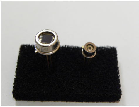
Figure 7.1: LEFT: the Si-Pin s1223 series from Hamamatsu, RIGHT: the Si-Pin s5973 series from Hamamatsu
