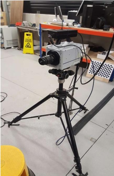
Figure 53: High speed imaging Fastcam SA4
