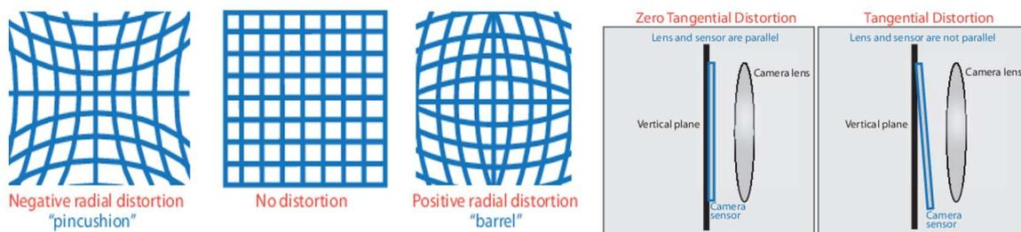
Figure 57: Radial and tangential distortion of the lenses (Matlab)
