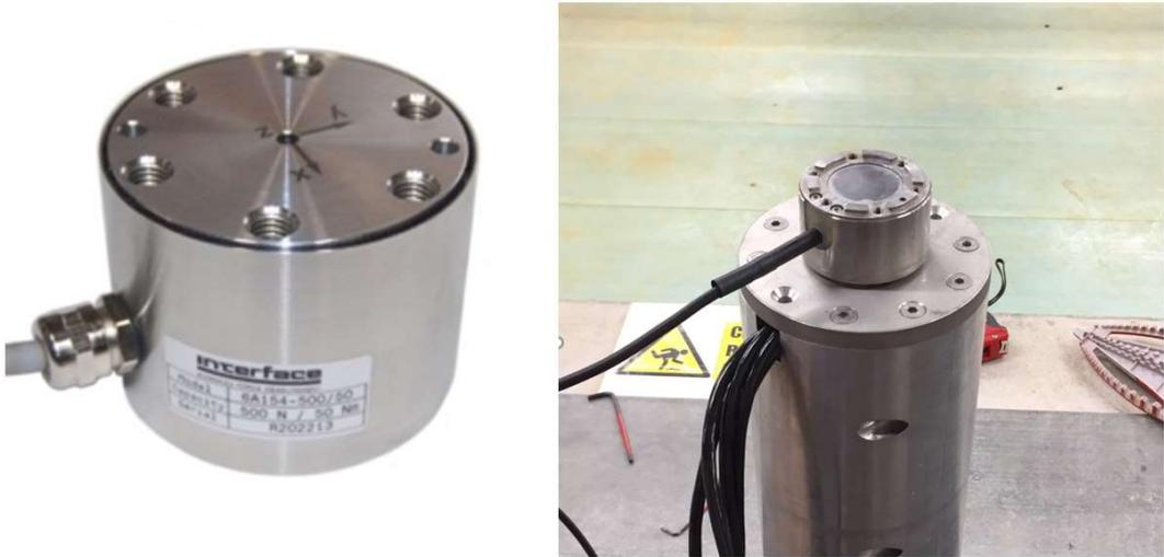
Figure 52: Load cell installation above the model
