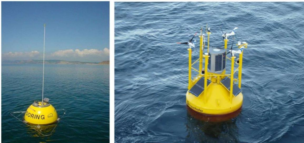
Figure 8: Directional waverider buoy (left), wind measurement (right)
