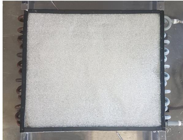
Figure 2.9: Finned heat exchanger in which the void between the fins is filled with silica gel grains.
