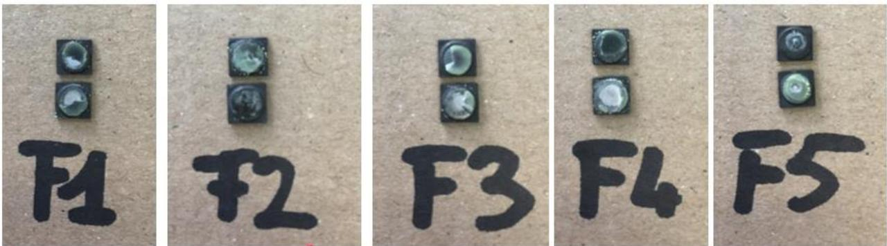
Figure 5.11: Fracture surfaces of samples belonging to batch F.
