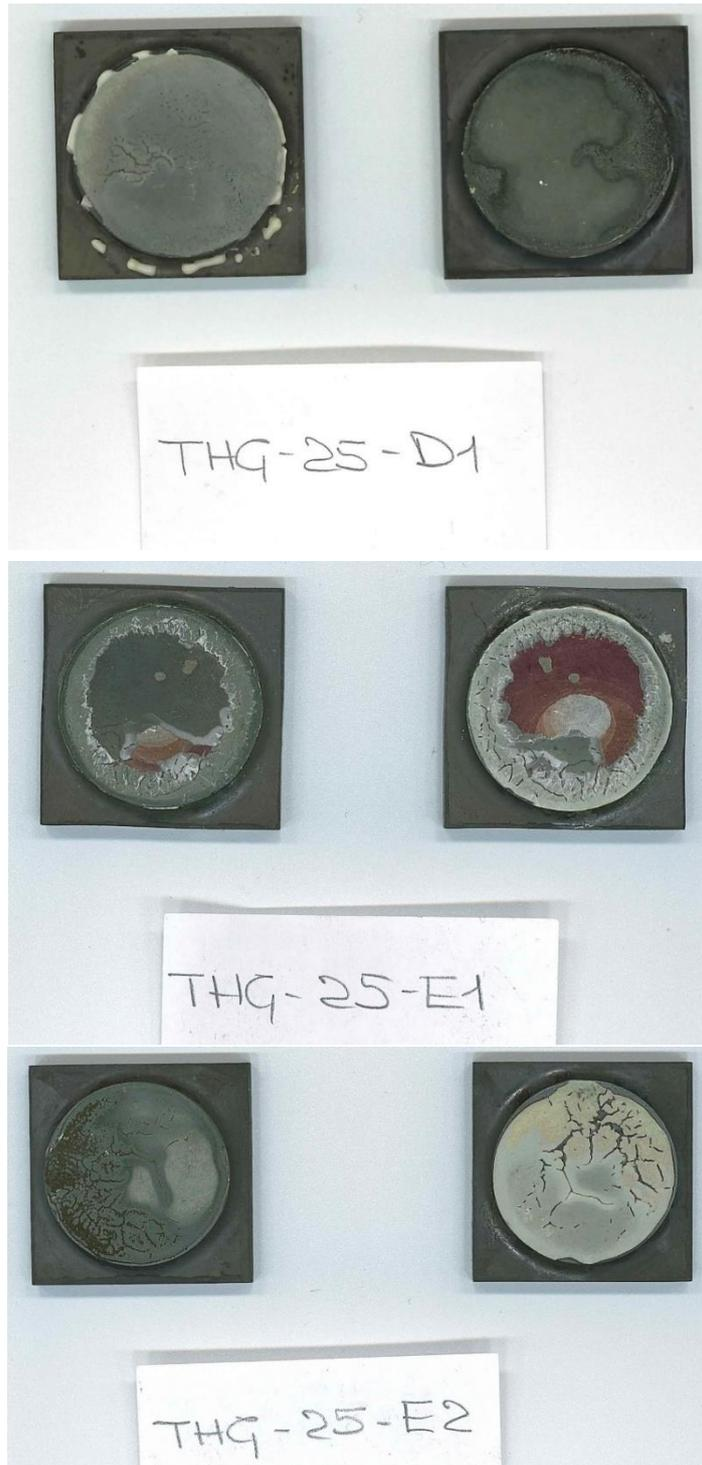
Figure 5.14: Fracture surfaces of THG 25 samples belonging to batches D and E.
