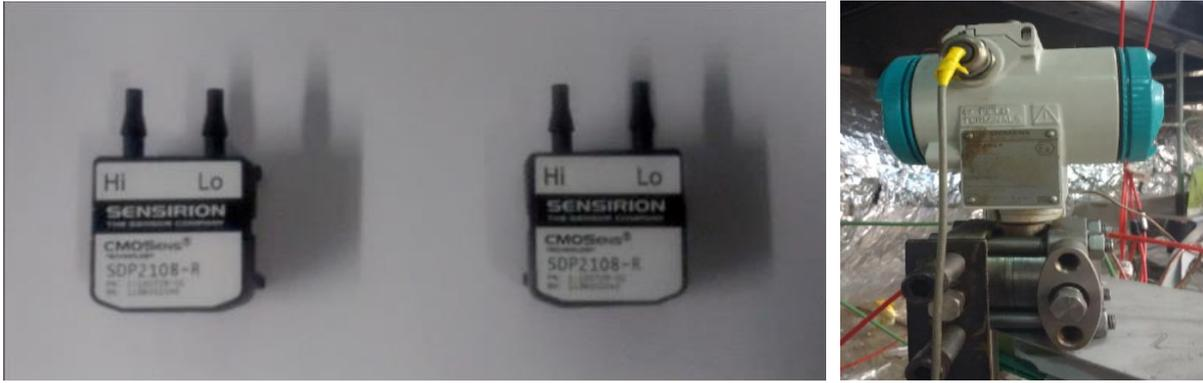
Figure 31 Pictures of the differential pressure sensors of the gas (left) and of the water(right)
