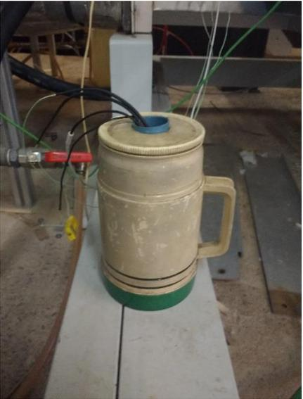
*Figure 29 Pictures of thermocouples type-K connected to the electronic cards(left) and the tank filled with water and ice with thermocouples immersed in(right)*
