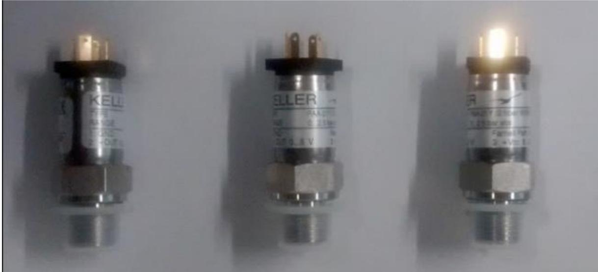
*Figure 30 Picture of the absolute pressure sensors*
