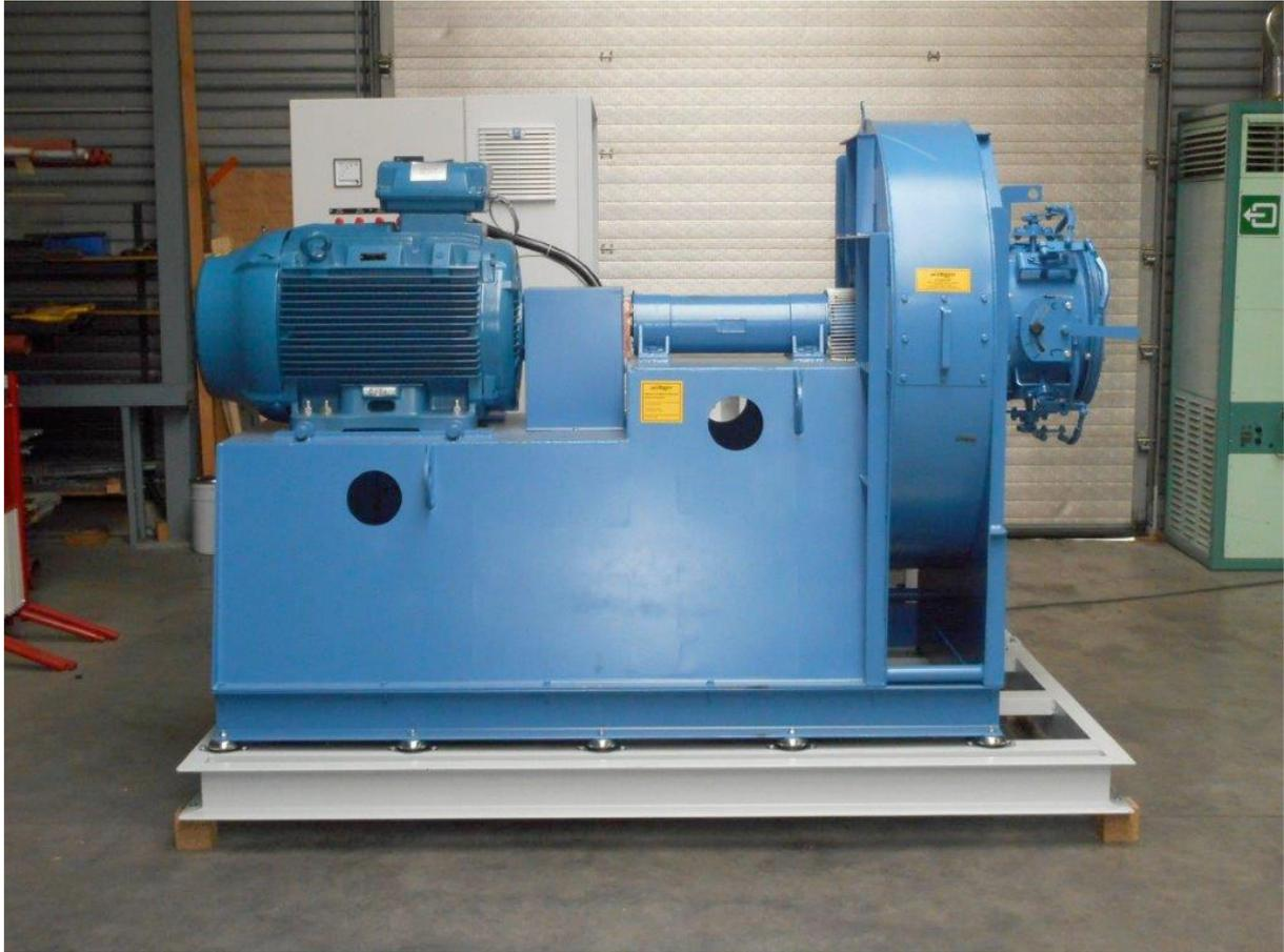
*Figure 11 Picture of the centrifugal air fan [1]*
