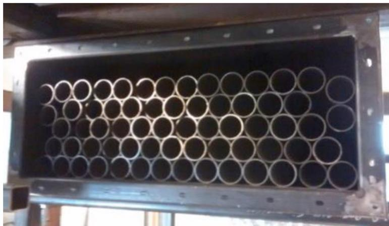
*Figure 14 Picture of the parallel tubes flow straightener [1]*
