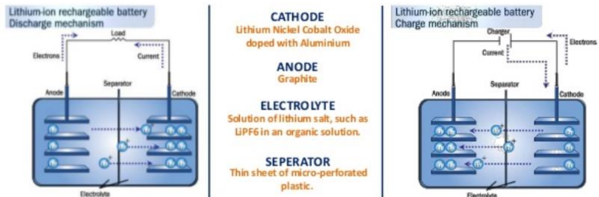
FIGURE 10. A LI-ION BATTERY TYPE AND FUNCTIONING
