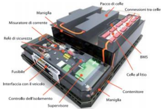
FIGURE 35. COMPONENTS OF A BATTERY PACK [24]
