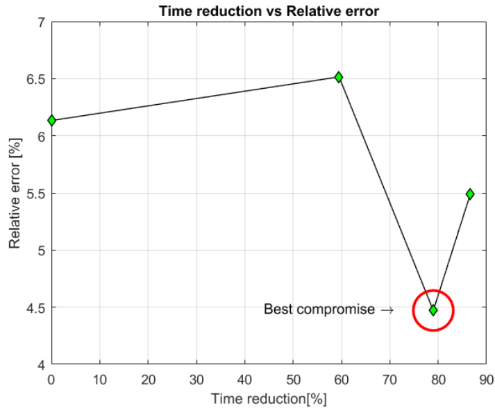
Figure 2.10: The percentage cpu time reduction with respect to the cartesian grid, versus the relative error with respect to the value presented in [9]. From this graph we can enlighten the best compromise grid that permit to reach a very high reduction in cpu time without increase the relative error.
